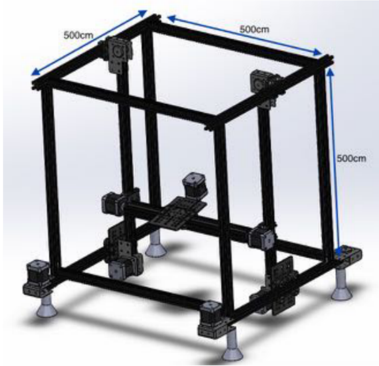
Figure 3: CAD Model of Gantry-Style Testbed [3]
