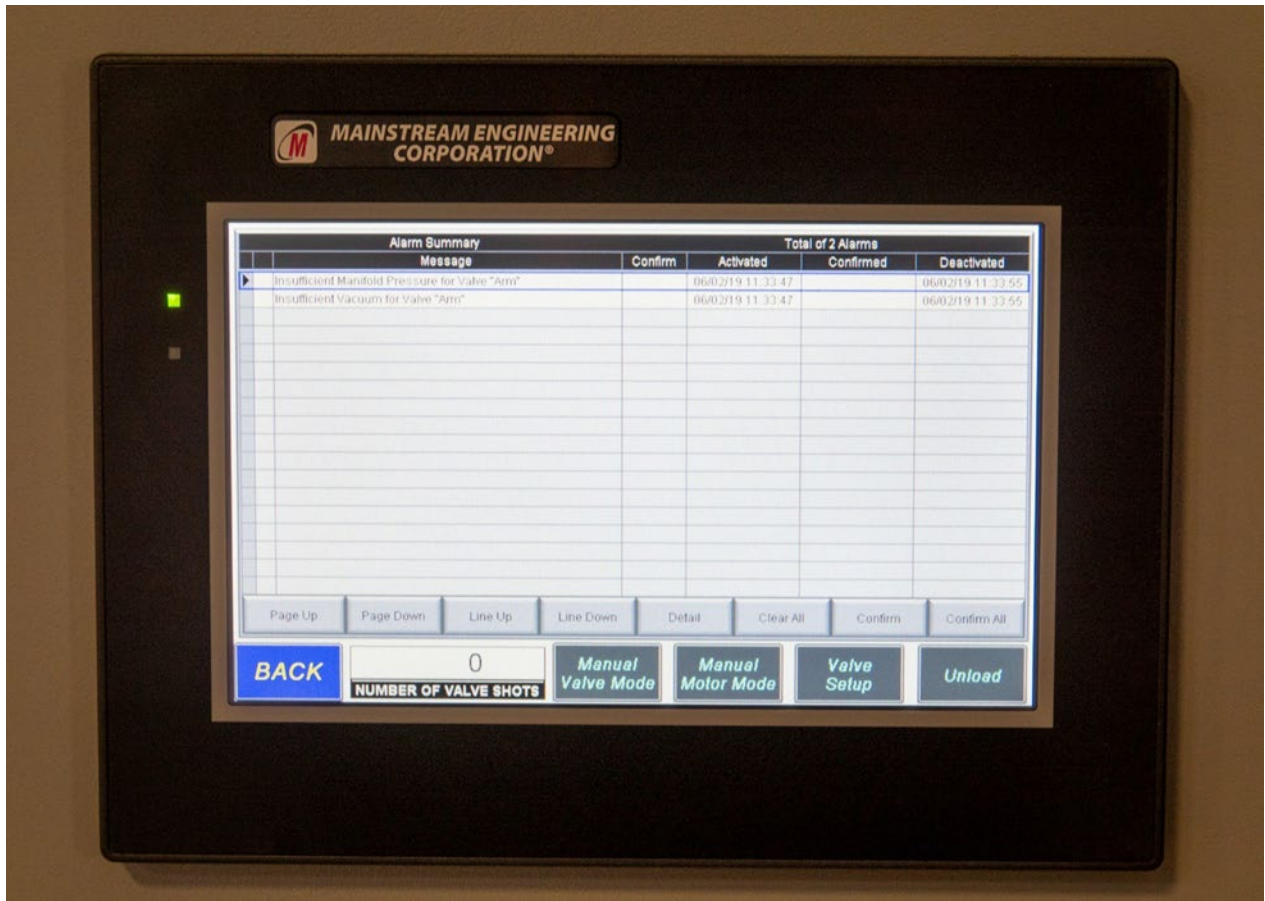
Figure 15. Alarm log screen
