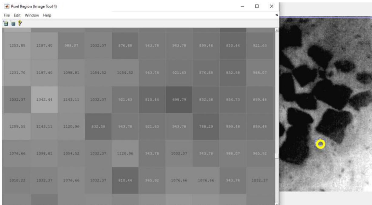
Figure 62. Pixels on the thermal image that have been converted to thickness values.
