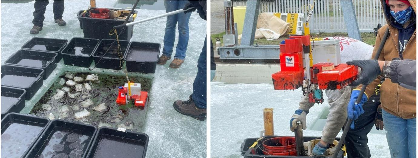
Figure 18. Example of sample processing for the tube sampler with emulsified (50/50) oil at 50  $\mu\text{m}$ .
