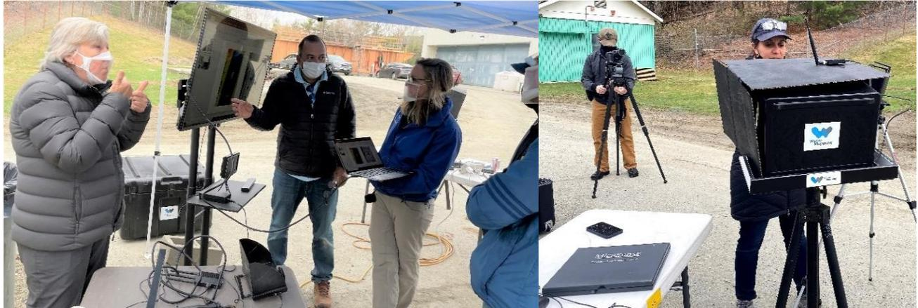
Figure 8. Left: Screens displaying the thermal and visual data in real time from the UAS. Right: Control base station that monitored the telemetry of the UAS.
