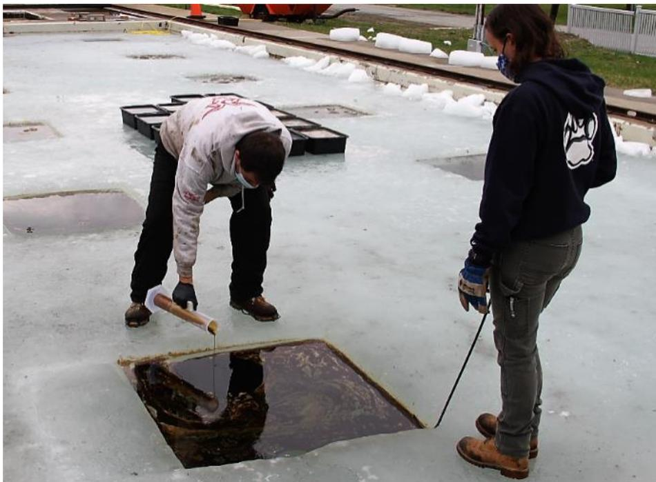
Figure 12. Adding controlled amounts of oil into squares to produce established thickness layers.
