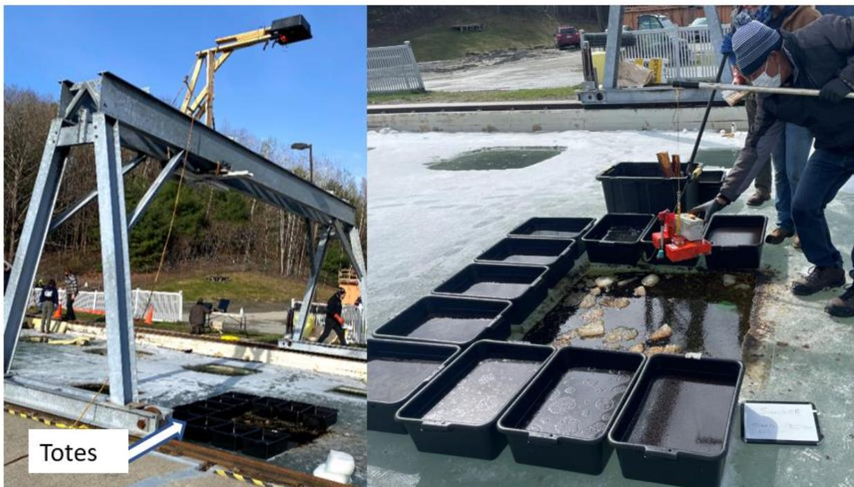
Figure 14. Setup for time-lapse study. Left: A-Frame with cameras; Right: setup of the totes with different thicknesses and oil types.
