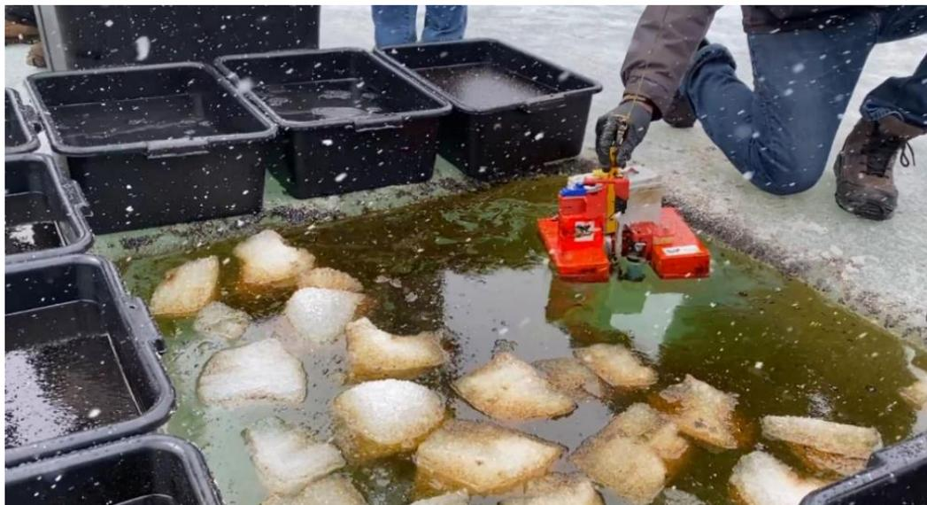
Figure 16. Tube sampler measuring oil thickness.
