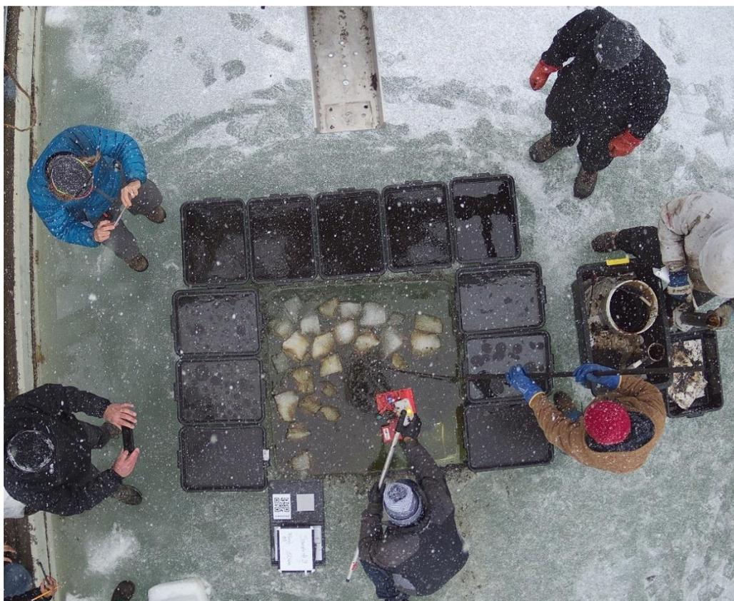
Figure 60. Top view from the multispectral imaging of a 1m x 1m square while the project team collected physical measurements of multiple thicknesses.
