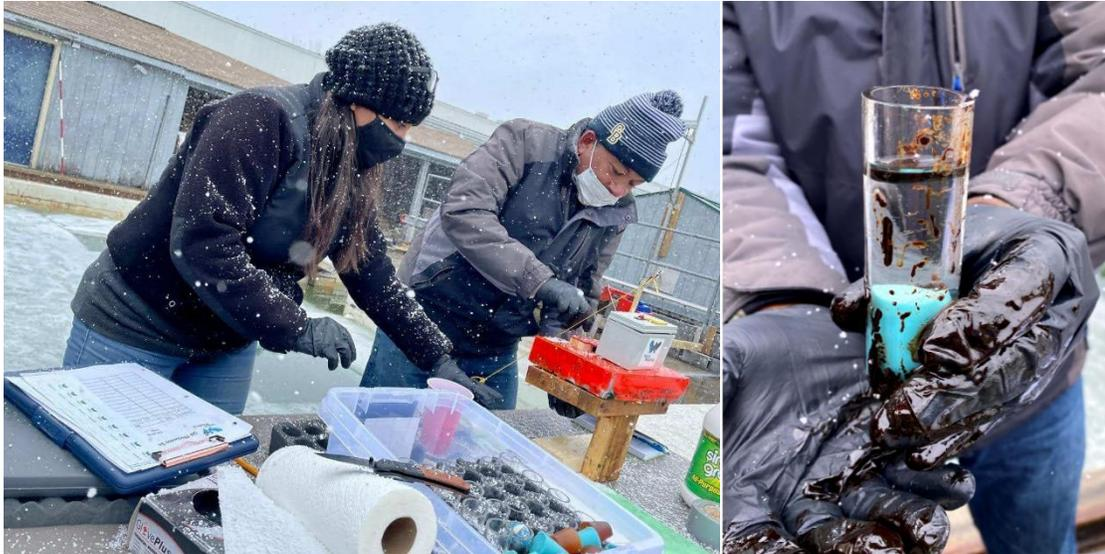
Figure 17. Processing the tube samples for oil thickness.
