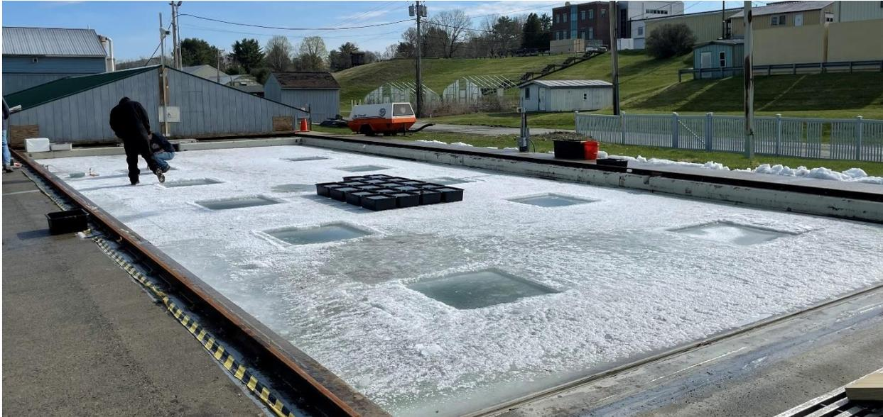
Figure 6. Ground view of the GRF tank with ice squares (1m x 1m) and black plastic totes for oil thickness calibration.
