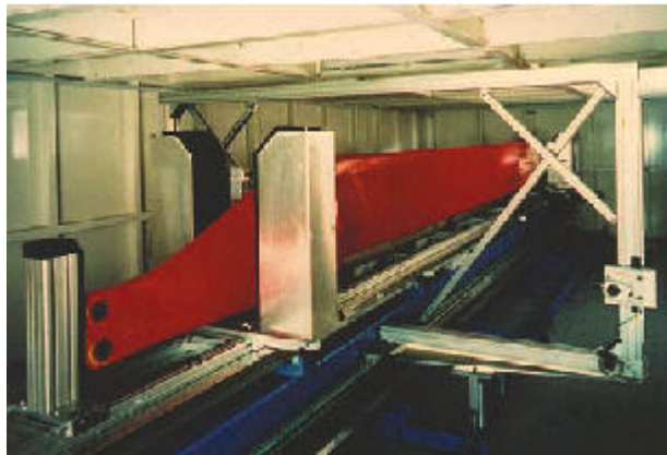
Figure 12. Shearography Applied to a Rotor Blade Inside a Vacuum Chamber. Source: Krupka (2003)
