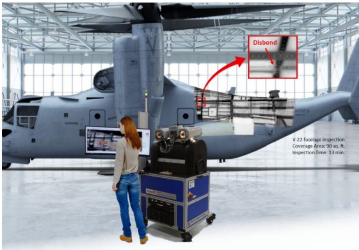
Figure 15. Large Area Inspection Concept as presented on the TWI website. Source: TWI, https://www.thermalwave.com/technology/ .
