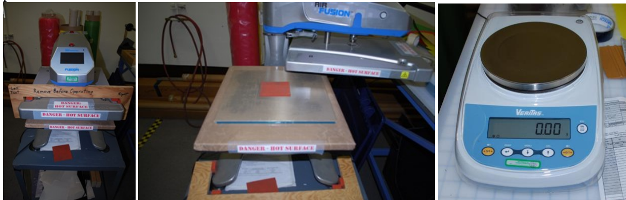
Figure 27 Modified ASTM D3531 Resin Flow test equipment used for quick evaluation of recycle prepreg processability
