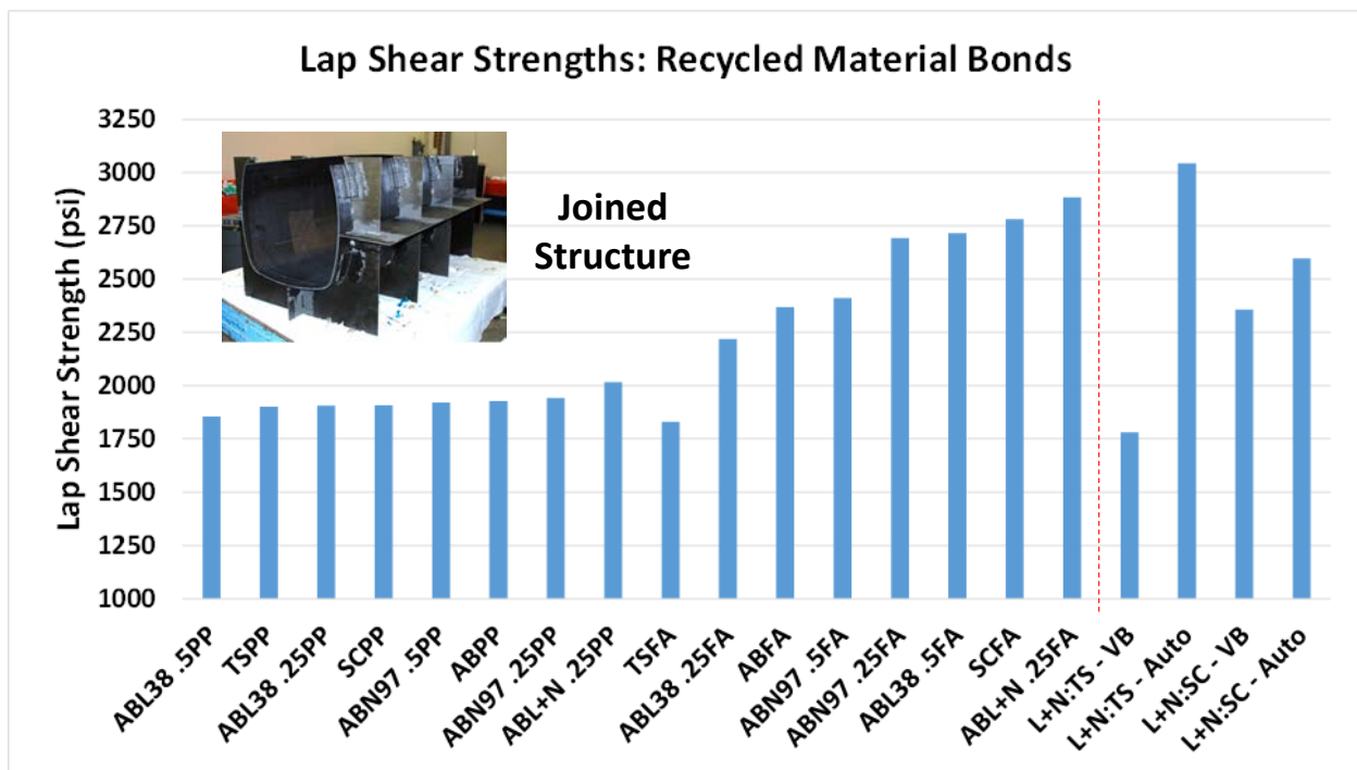
Figure 17: Lap shear results determining range of joint strengths of likely processing variability
