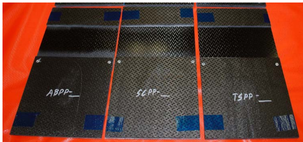
Figure 15: Lap shear bonding trial panel configuration with doublers to align test load axis
