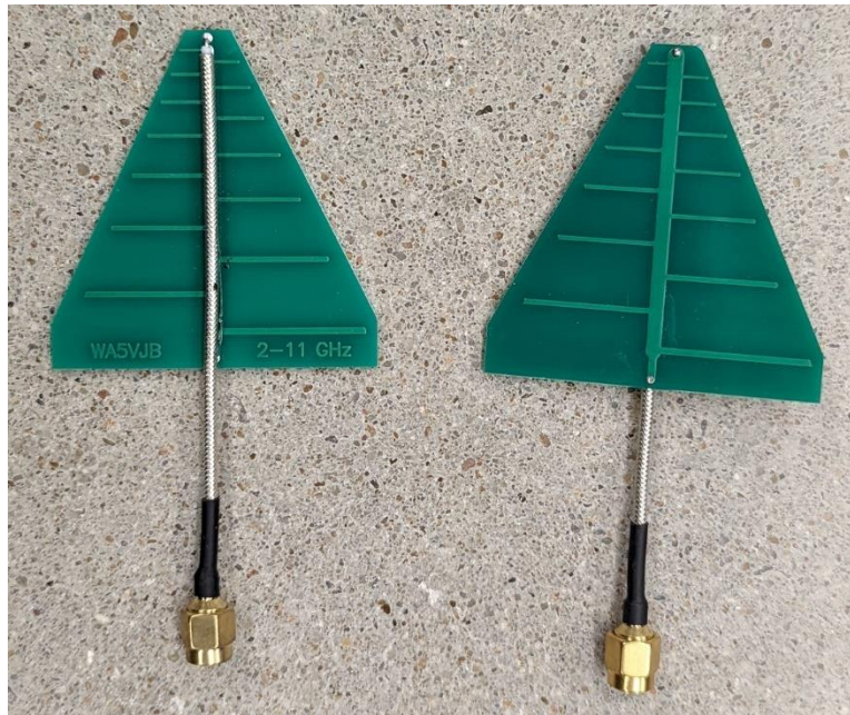
Figure 11: 2-11 GHz Planar Log-periodic antennas
