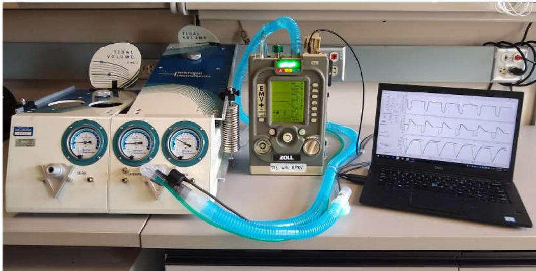
Figure 9: Photograph of the ZOLL EMV+<sup>®</sup> 731 Series ventilator with prototype firmware, delivering an airway pressure release ventilation (APRV) waveform to a Michigan Instruments test lung.
