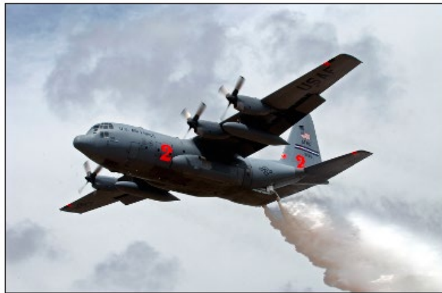
Figure 6. C-130 with MAFFS. “Modular Airborne Firefighting System,” Wikipedia Foundation, last modified January 9, 2021, https://upload.wikimedia.org/wikipedia/commons/5/5e/C-130_Waterdrop.jpg .
