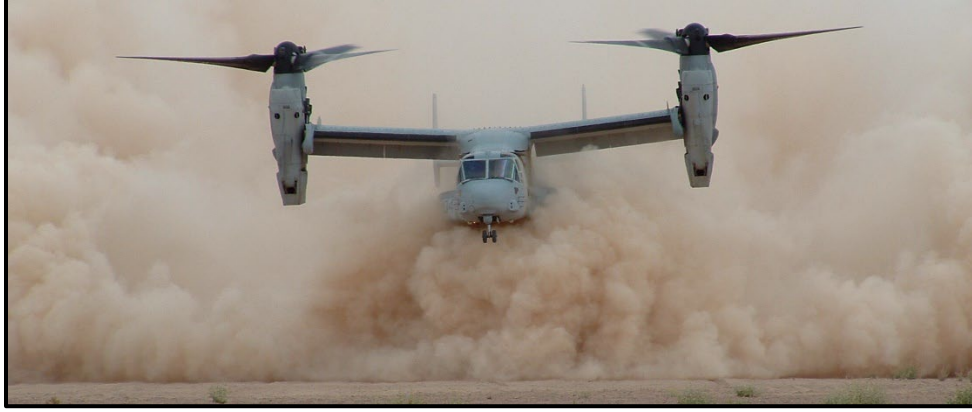
Fig. 1 Marine Corps MV-22 operating in brownout conditions (Harrington 2007)
