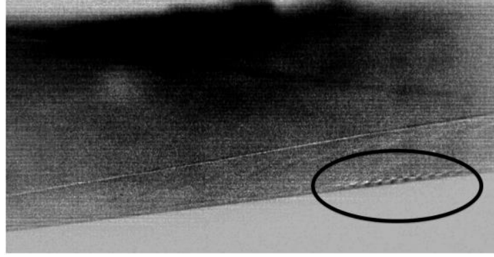
Figure 10 Focused schlieren image of Mach 10 boundary layer, Re = 2 \times 10^6/ft . Adapted from [36].
