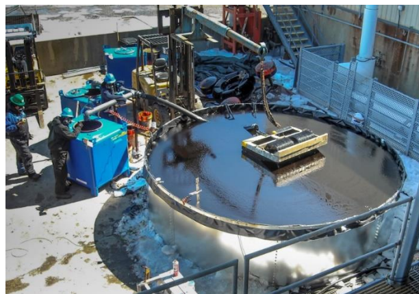
Figure B-7. Skimmer test with dilbit in Ohmsett's fresh water tank.
