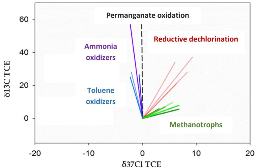
Figure 8. Dual element C-Cl trends in aerobic cometabolic biodegradation of TCE contrasted with reductive dechlorination. Isotope ratios are normalized to zero for the initial TCE isotope composition. Figure modified after Gafni et al., 2020.
