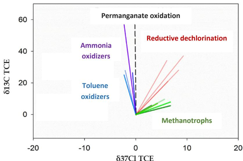
Figure 3. Dual element C-Cl trends in aerobic cometabolic biodegradation of TCE contrasted with reductive dechlorination. Isotope ratios are normalized to zero for the initial TCE isotope composition. Figure modified after Gafni et al. (Chemosphere, Volume 242, March 2020, 125130)
