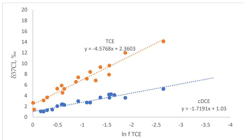
Figure 4. Rayleigh-type plot of chlorine isotope data in ZVI degradation of TCE. The early product depletion of cDCE can be read from the regression intercepts. TCE reactant is isotopically identical as in the data set shown in Figure 7.
