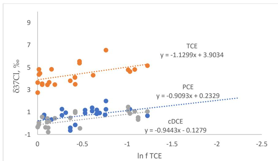
Figure 6. Rayleigh-type plot of chlorine isotope data degradation of PCE by *Desulfuromonas michiganensis*, Bio-Dechlor Inoculum (BDI), *Geobacter lovleyi*. The early product depletion of cDCE and the early product enrichment of TCE can be read from the regression intercepts. The same PCE reactant was used in all experiments.
