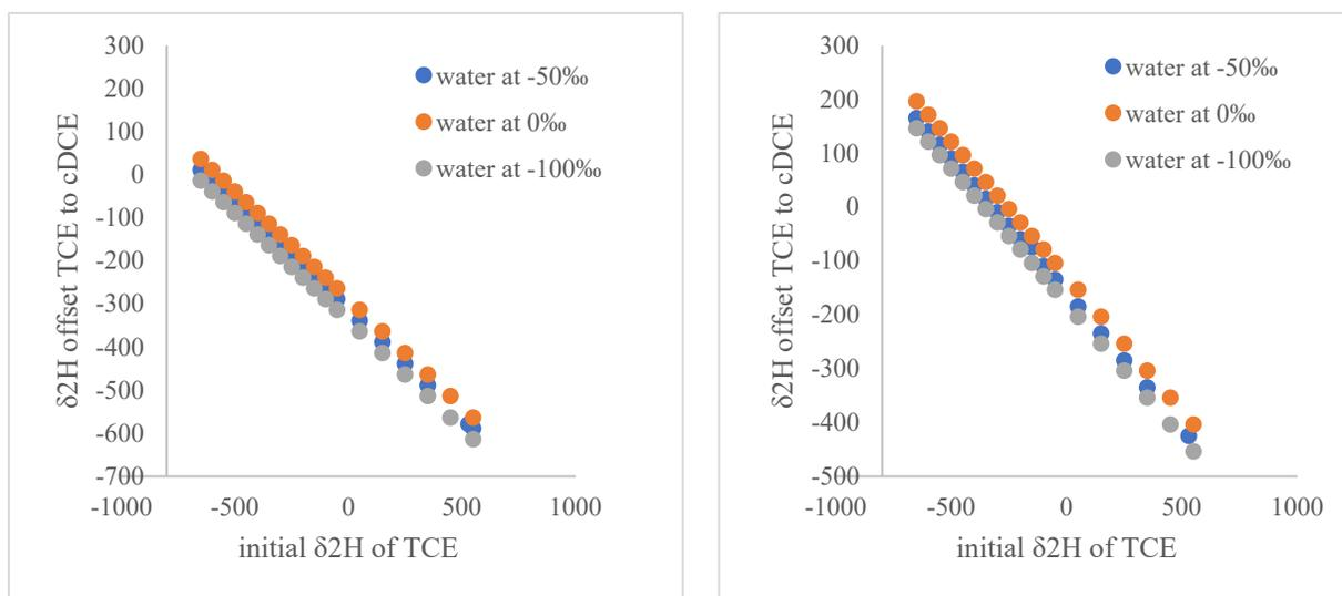
Figure 2. Offsets of  $\delta^2\text{H}$  between TCE and cDCE in abiotic (A) and biological (B) reductive dechlorination. Panel B is based on isotope data in degradation of PCE to cDCE by *Desulfuromonas michiganensis* experiment (see the following section). Net value of  $\delta^2\text{H}$  of cDCE is obtained by subtracting the value of offset (Y axis) from the corresponding  $\delta^2\text{H}$  of TCE (X-axis).
