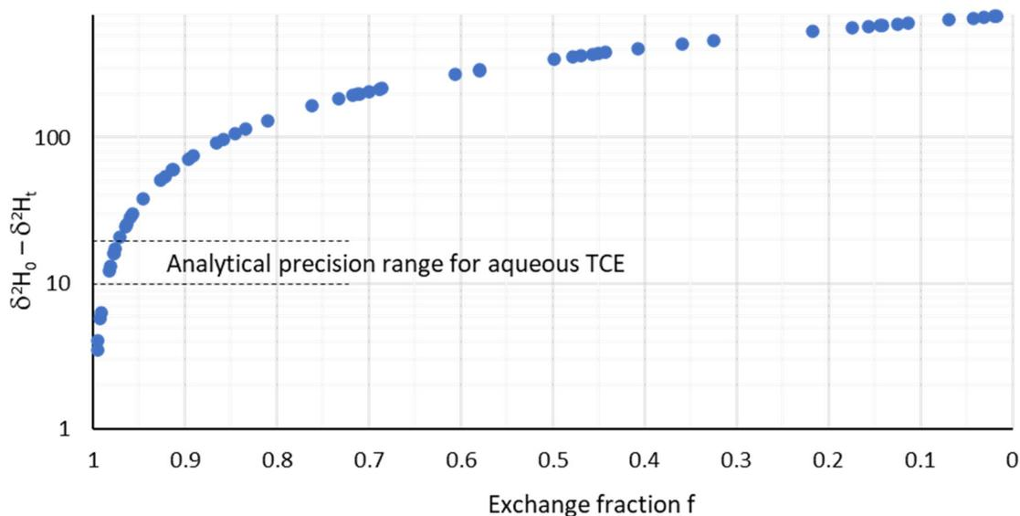
Figure S1. Net change of  $\delta^2\text{H}$  of TCE as a function of exchange fraction, based on the results from exchange with non-labeled water, at  $\delta^2\text{H}$  difference between water and TCE of 600 ‰. The results shown are for all experiments with TRIS buffer. The precision range is based on the low-temperature chromium method applied to relatively dilute samples with purge and trap preconcentration.
