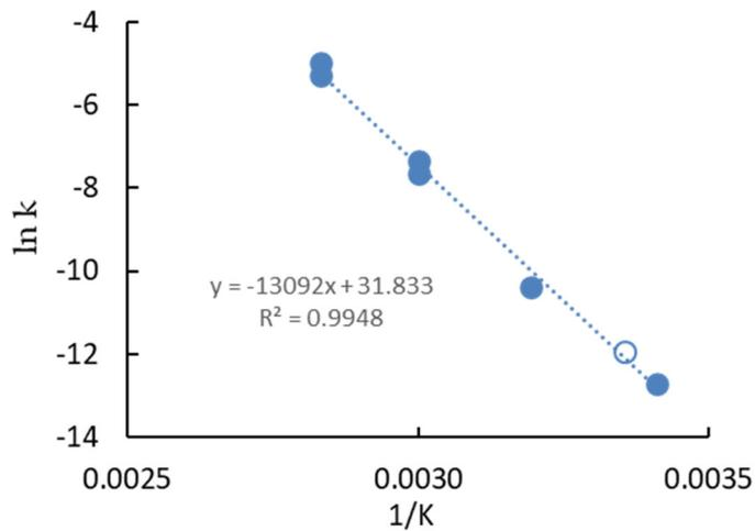
Figure 3. Arrhenius plot of data normalized to pH=7, including those reported by Gabričević et al., indicated by the hollow marker. See Table 1 for numerical data.
