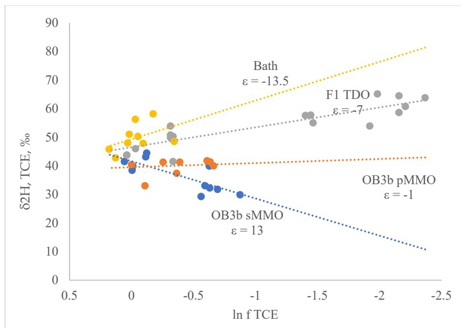
Figure 9. Rayleigh-type plot of hydrogen data from aerobic biodegradation. Note that the regression slope except in OB3b sMMO and F1 TDO are not statistically significant.
