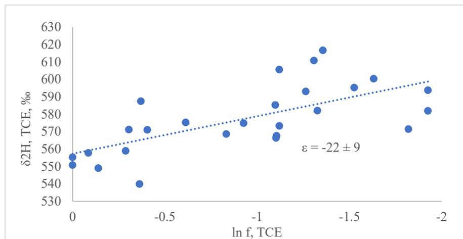
Figure 1. Rayleigh-type plot of TCE degradation on ZVI. X axis represents the natural log of TCE fraction remaining. Data represent four rounds of degradation experiments.
