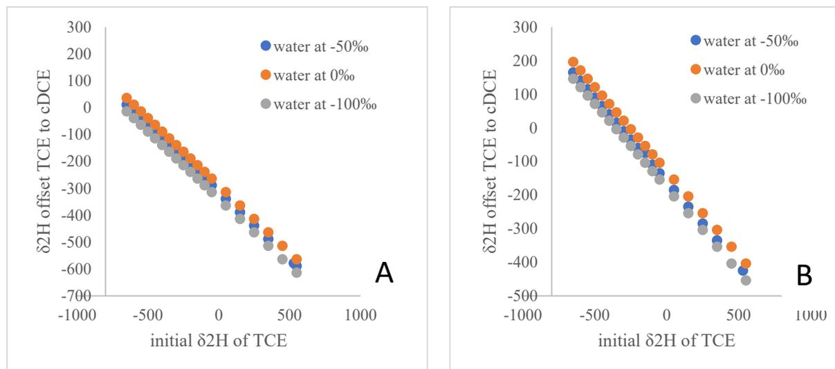
Figure 3. Offsets of  $\delta^2\text{H}$  between TCE and cDCE in abiotic (A) and biological (B) reductive dechlorination. Panel B is based on isotope data in degradation of PCE to cDCE by *Desulfuromonas michiganensis* experiment (see the following section).
