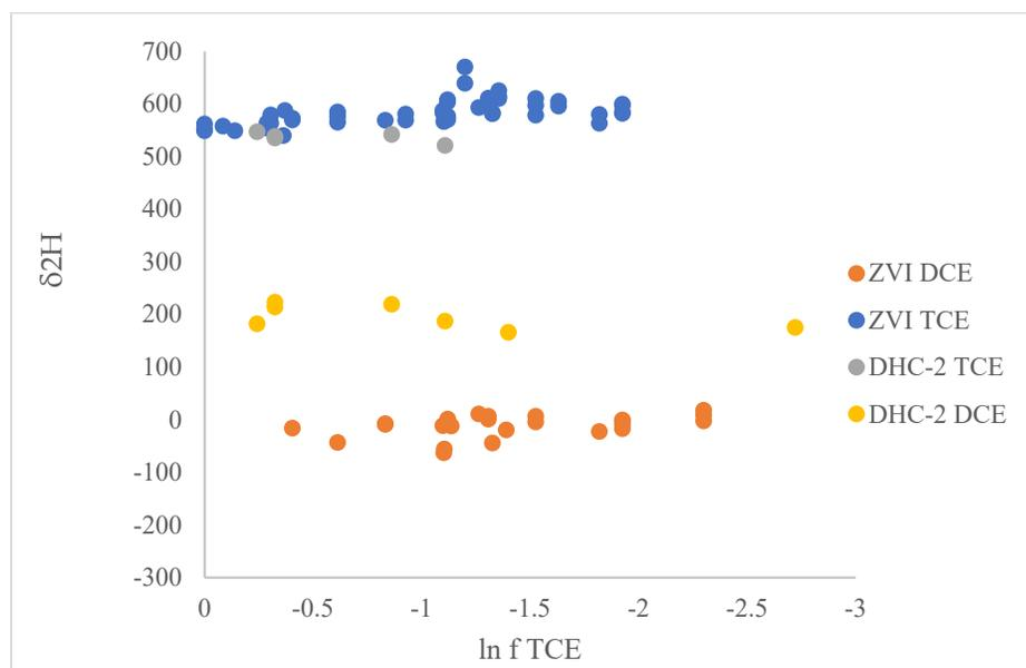
Figure 1. Hydrogen isotope ratios of TCE and cDCE vs remaining mass of TCE, in degradation of TCE on ZVI and in biodegradation of identical TCE by *Dehalococcoides mccartyi* strain 195. ZVI data represent four rounds of degradation experiments. The same lot of TCE was used in both experiments.
