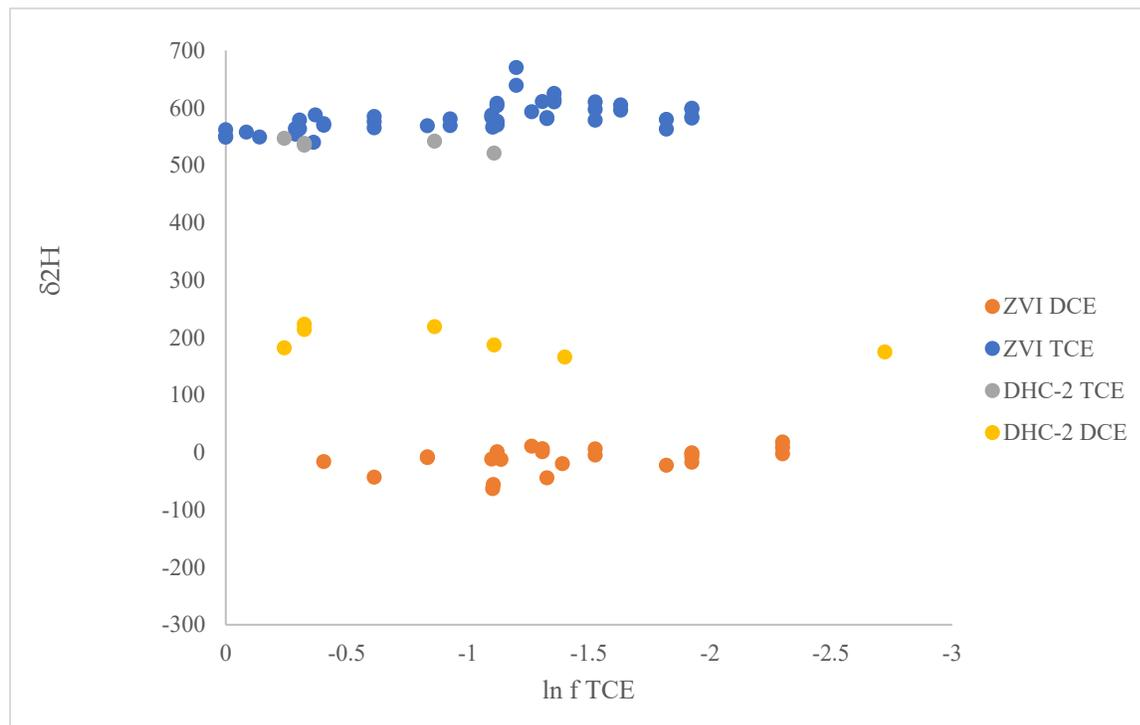
Figure 2. Hydrogen isotope ratios of TCE and cDCE vs remaining mass of TCE, in degradation of TCE on ZVI and in biodegradation of identical TCE by *Dehalococcoides mccartyi* strain 195. ZVI data represent four rounds of degradation experiments.
