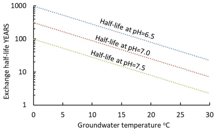
Figure 4. Half-lives of the exchange as a function of groundwater pH and temperature.
