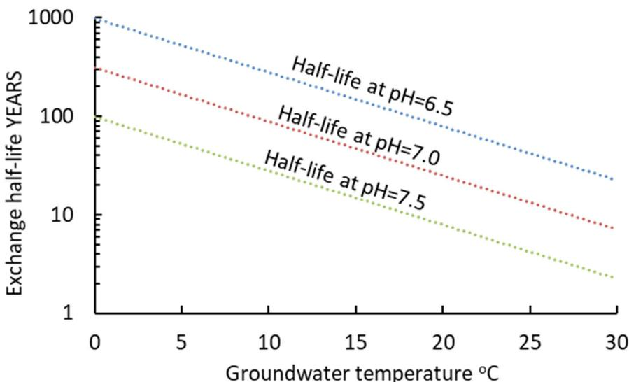
Figure 4. Hydrogen exchange half-lives as a function of aquifer pH and temperature. The rates are based on kinetic experiments performed as part of this project.
