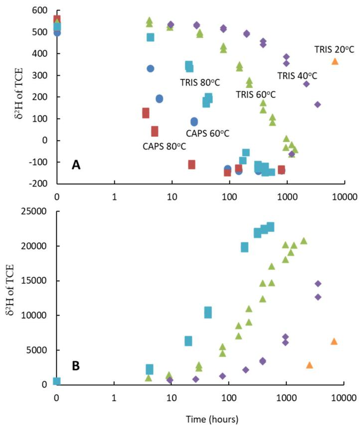
Figure 1. Evolution of  $\delta^2\text{H}$  of TCE over equilibration with (A) water at  $\delta^2\text{H} = -50\text{‰}$ ; and (B) water at  $\delta^2\text{H} = +26500\text{‰}$ . Time  $T=0$  hrs is recorded as 0.1 hrs, to permit the use of the log scale of the time axis. Data subsets are labeled by the respective pH buffer and temperature.
