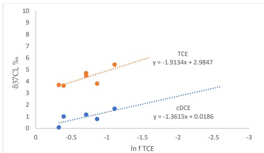
Figure 7. Rayleigh-type plot of chlorine isotope data in degradation of TCE by *Dehalococcoides mccartyi*. The early product depletion of cDCE can be read from the regression intercepts. TCE reactant is isotopically identical as in the data set shown in Figure 4.
