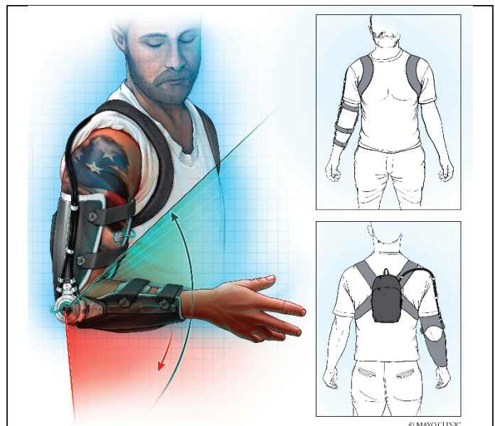
Figure 1. Design concept for the myoelectrically-controlled power-assist upper-extremity exoskeleton (powered exoskeleton).
