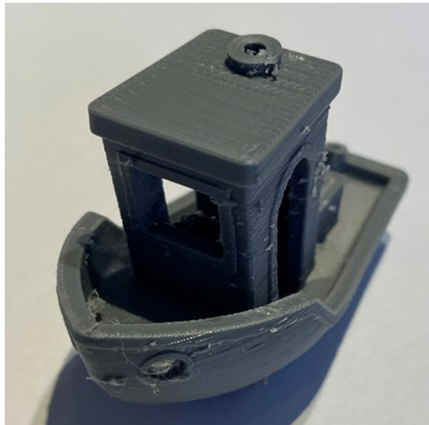
Fig. 7 3D Benchy with PVA removed
