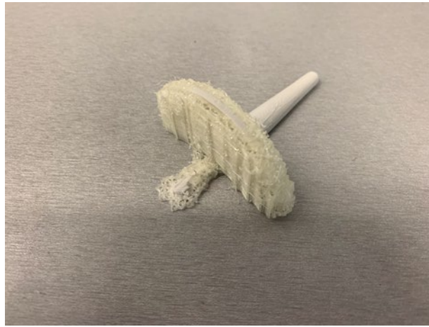
Fig. 8 Jet formation with PVA support
