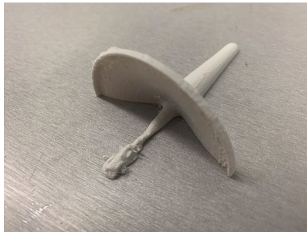
Fig. 9 Jet formation with PVA removed
