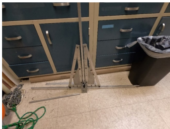
Figure ES-2. The Modified Multisampler Anchor without PE Sheets in the Laboratory.
