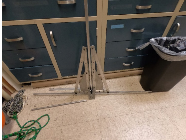
Figure 4. The Modified Multisampler Anchor Without PE Sheets in the Laboratory
