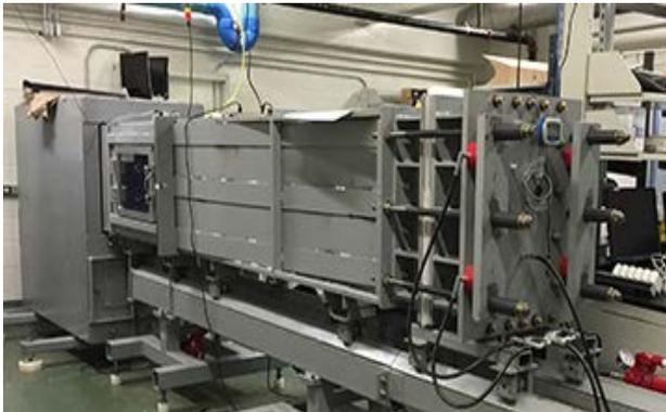
Fig. 1. The Advanced Blast Simulator (ABS)
