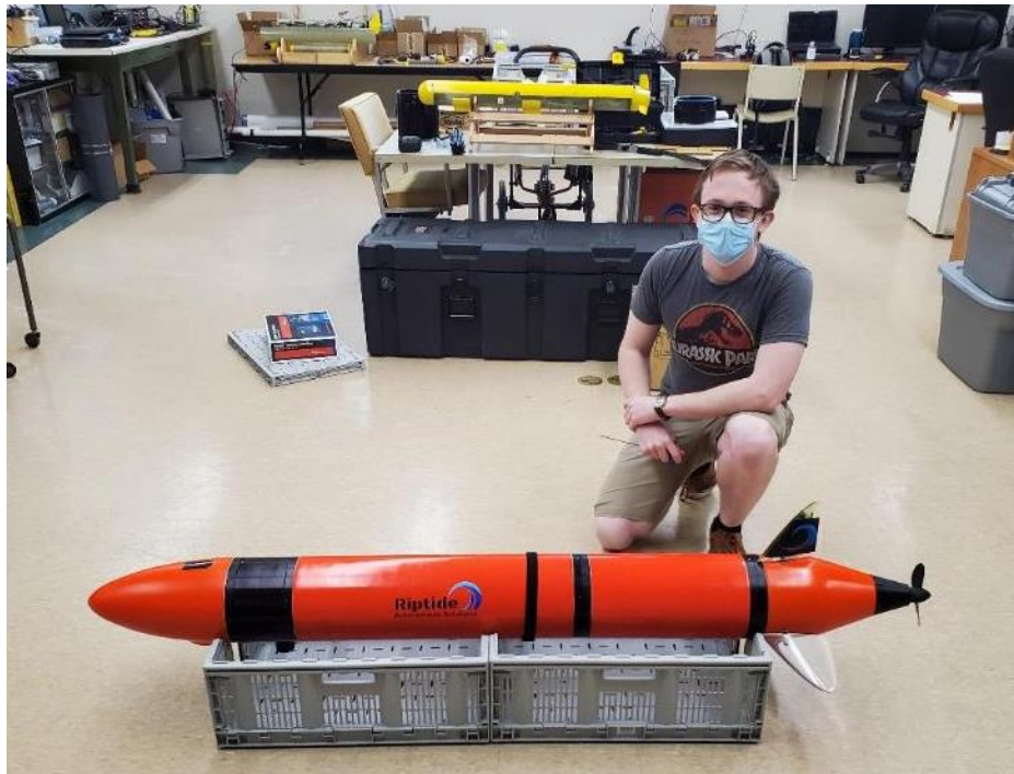
Figure 1. UI Riptide assembled with instrumentation and battery sections.
