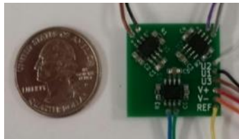
Figure 4. 3" ball sensor with embedded UI pre-amplifier.
