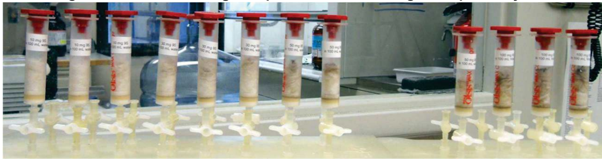
Figure 6. Appearance of 150 mg WAX SPE cartridges packed with glass wool to half the height of the cartridge barrel. Picture taken after passing aqueous samples containing 10, 30, 50 and 100 mg in triplicate from left to right, respectively.
