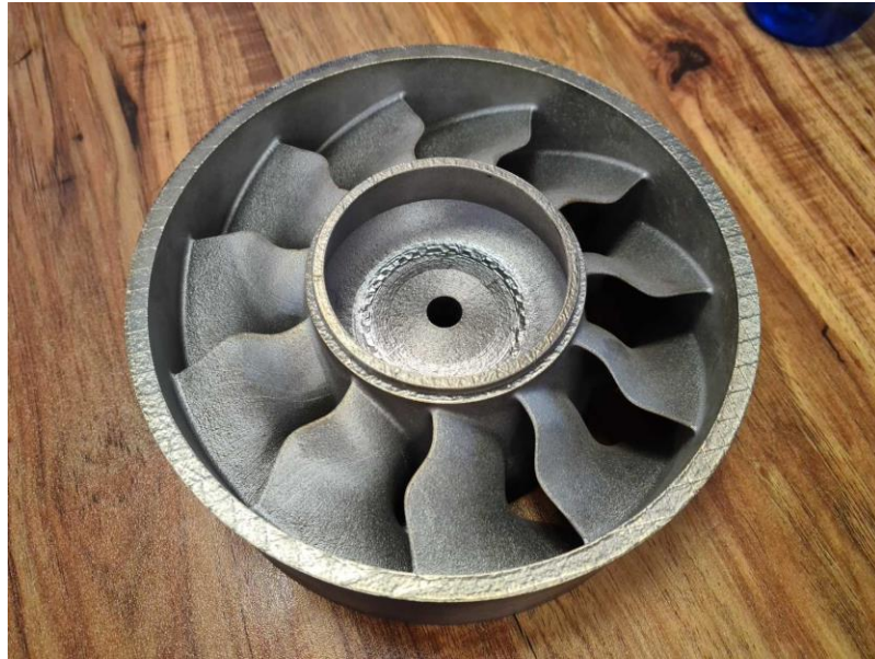
Figure 29: Additively Manufactured highly twisted fan
