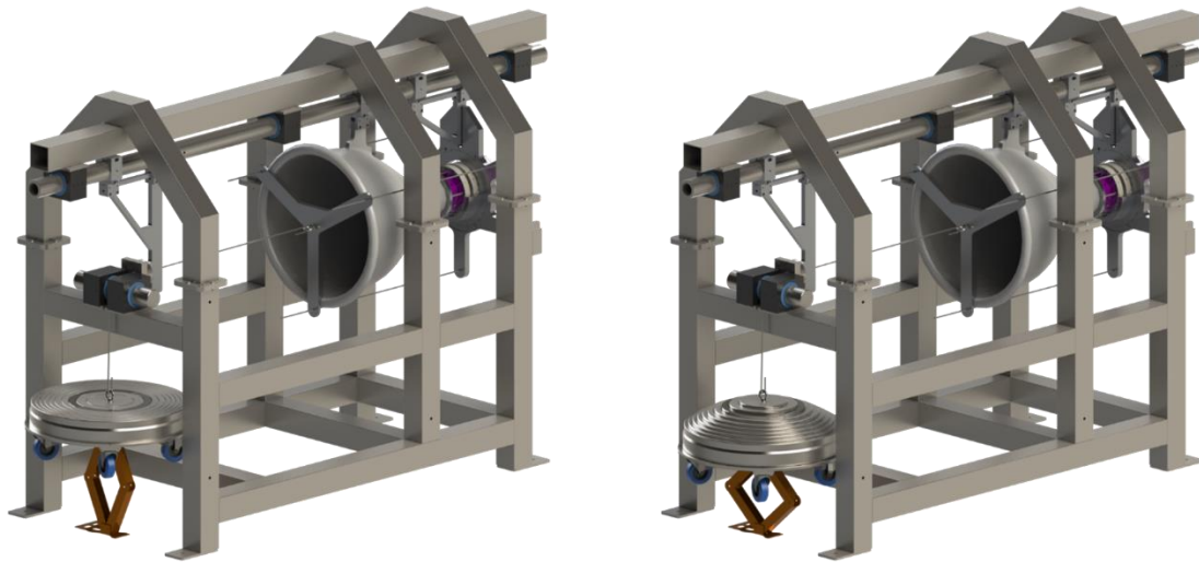
Figure 14: Calibration process: open jack – no load (left), closed jack - 200kg load (right)
