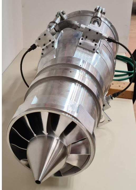
Figure 31: Assembled turbofan engine (without inlet)
