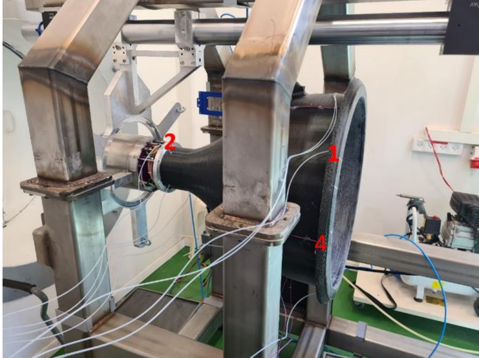
Figure 32: Probe location on test stand
