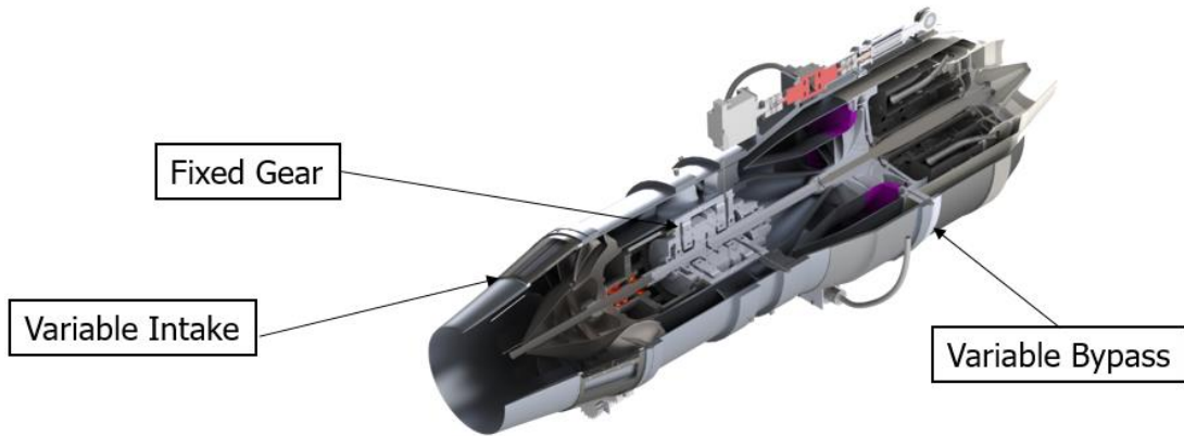
Figure 25: Adaptive cycle engine final assembly design
