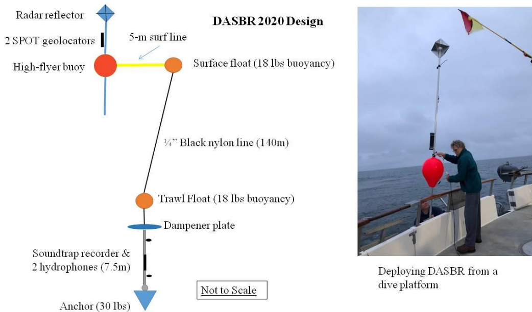
Figure 2. Diagram of the DASBR highlighting each of the components, including the Soundtrap recorder and two hydrophones.
