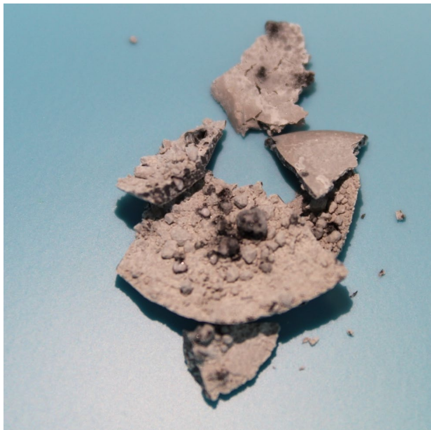
Figure 29. \text{HfB}_2 held at 1000 °C for 10 hours. There is no physical difference compared to Figure 25.
