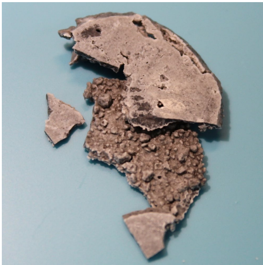
Figure 35. HfB 2 held at 1300 °C for ten hours.
