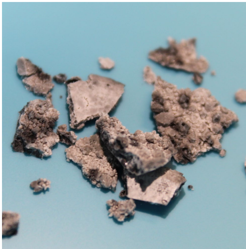
Figure 31. \text{HfB}_2 held at 1000^\circ\text{C} for 100 hours. No major physical changes to the sample.
