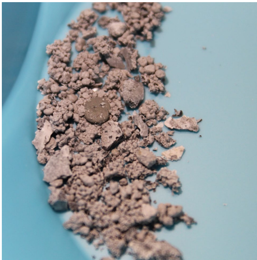
Figure 33. \text{HfB}_2 held at 1300 °C for 1 hour. There are no noticeable physical changes compare from the 1000°C heated samples.
