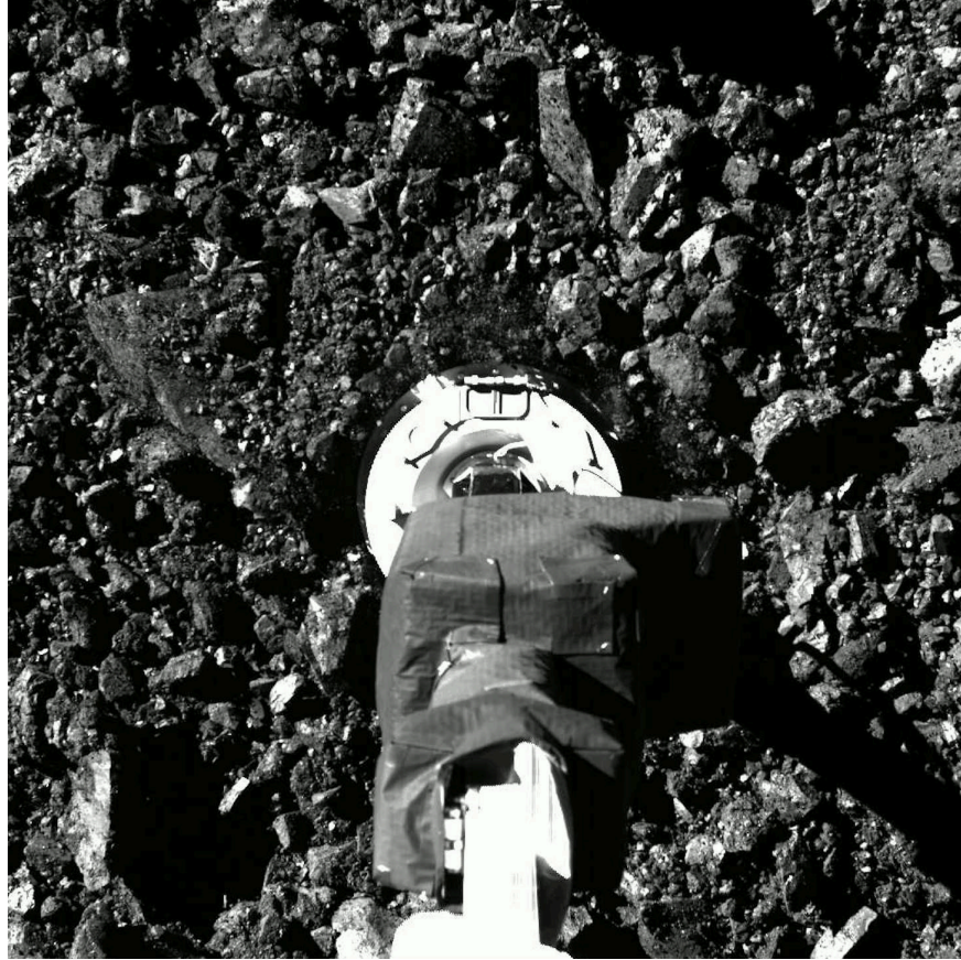
Figure 18. Image of OSIRIS-REx Touchdown on Bennu's Surface at Sample Site Nightingale 160
