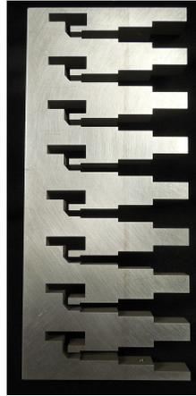
Fig. 6 — Fabricated column element using EDM
