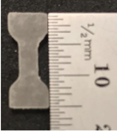
Fig. 1 Sample geometry prior to tensile testing
