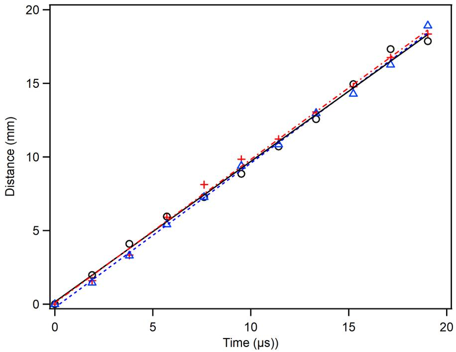
**Fig. 12** Flame-speed average velocity calculations for pSi produced by anodic etching of p-type Si wafer from image in Fig. 10a) blue triangles, 10b) red crosses, 10c) black circles; linear fits are shown
