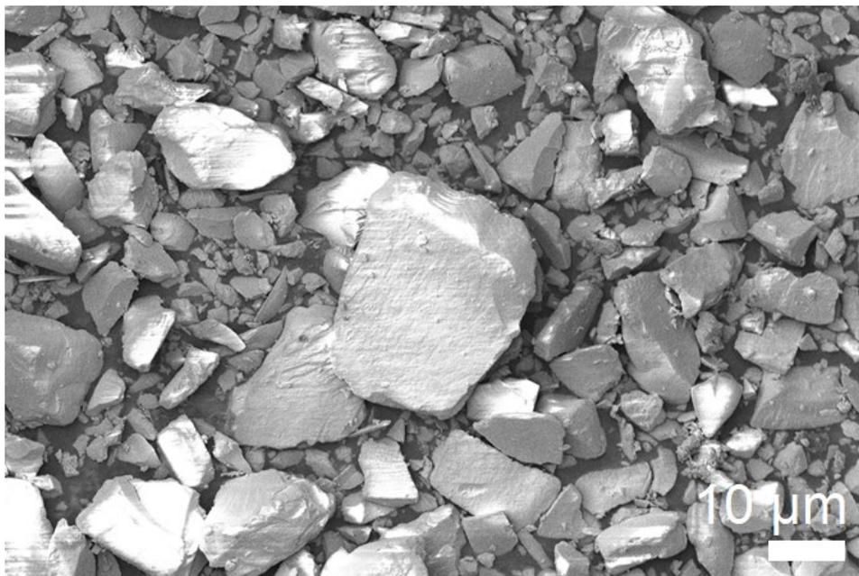
**Fig. 3** SEM image of pSi particles produced by anodic etching of p-type Si wafer
