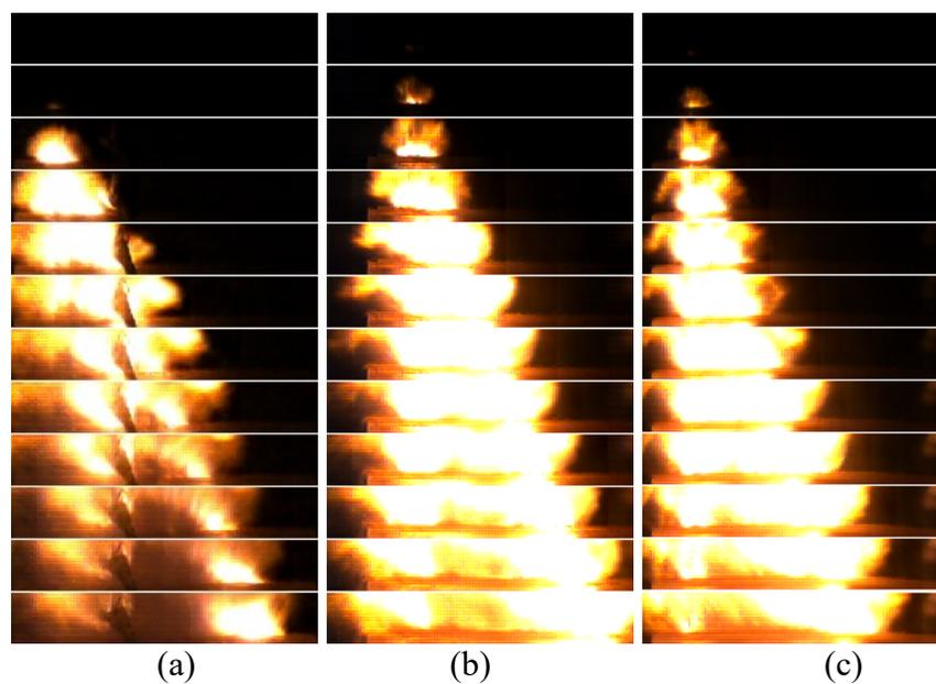
**Fig. 9** Flame propagation frame captures for pSi from Mg<sub>2</sub>Si
