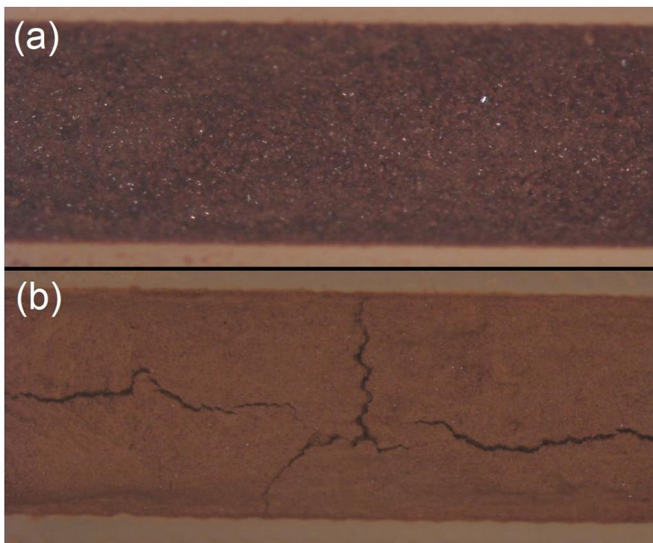
**Fig. 13** Microscope image of packing behavior of pSi produced (a) by anodic etching of p-type Si wafer and (b) from Mg<sub>2</sub>Si
