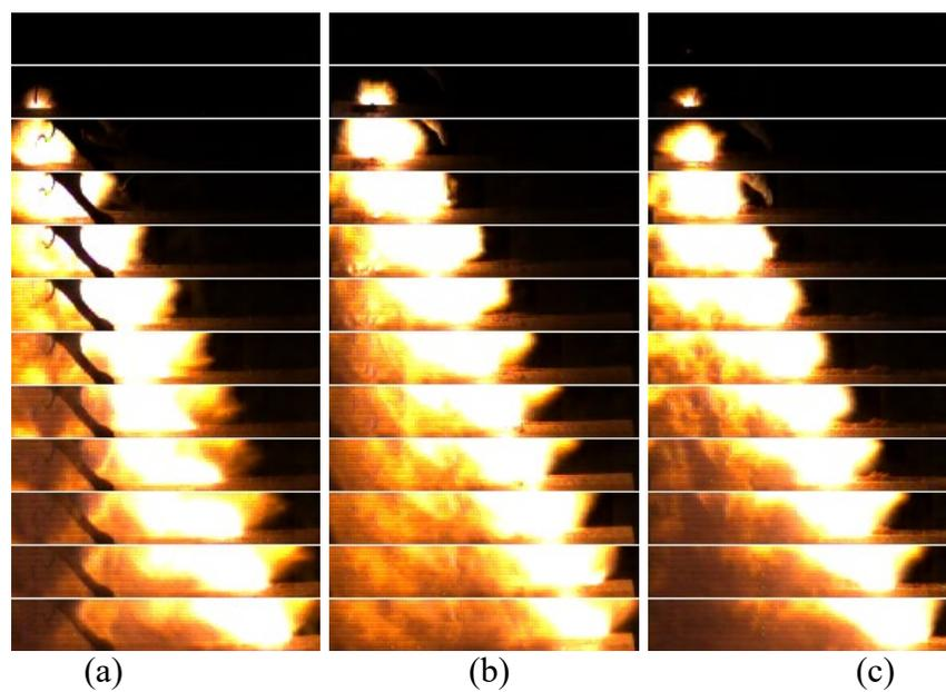
**Fig. 10** Flame propagation frame captures for pSi produced by anodic etching of p-type Si wafer
