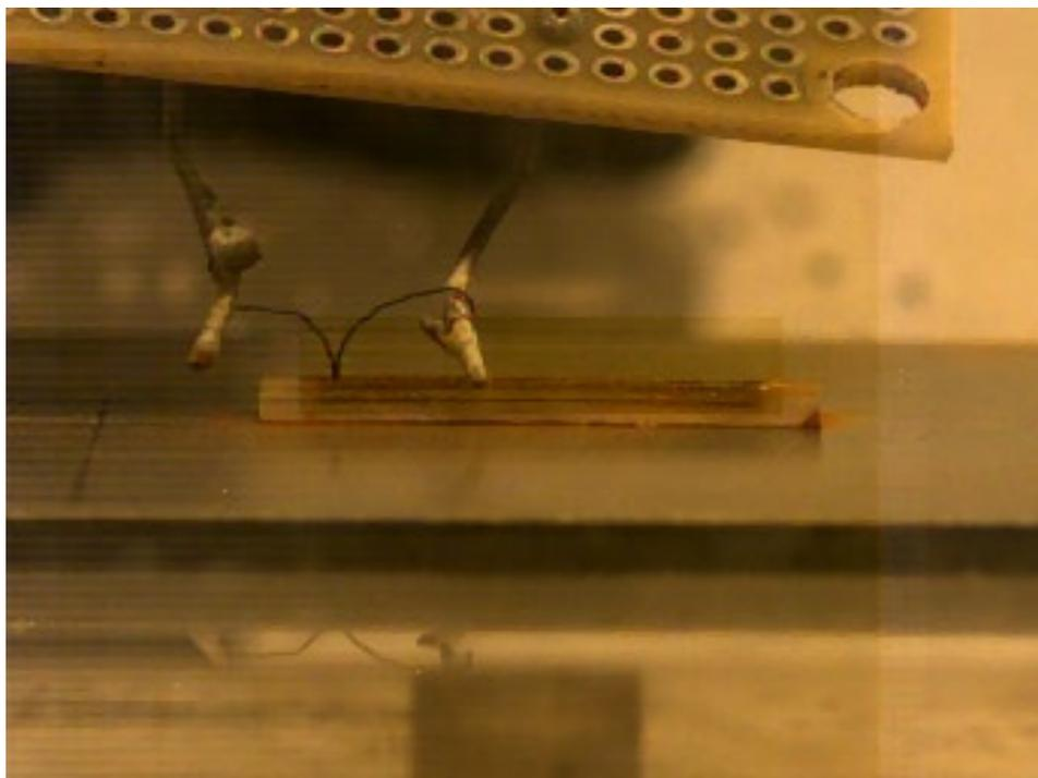
**Fig. 8** Representative reference photo of a pSi/NaClO<sub>4</sub> sample prior to ignition
