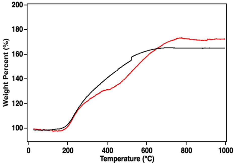
Fig. 7 Thermal gravimetric analysis plot of pSi (black) from Mg<sub>2</sub>Si and (red) by anodic etching of p-type Si wafer. The heating rate was 20 °C/min in air.
