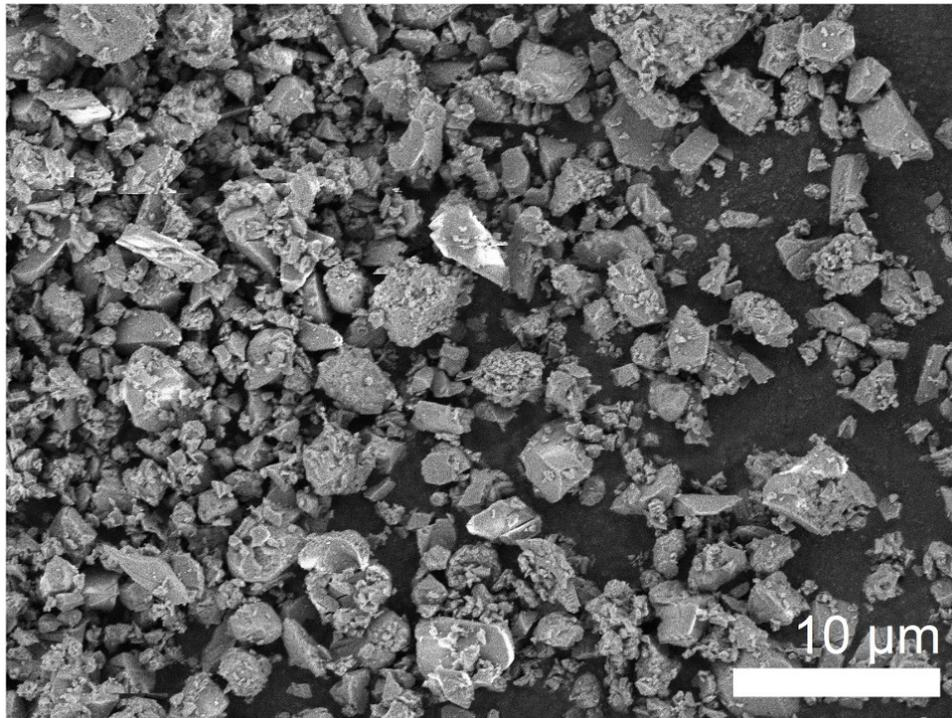
**Fig. 2** SEM image of pSi particles produced from  $\text{Mg}_2\text{Si}$
