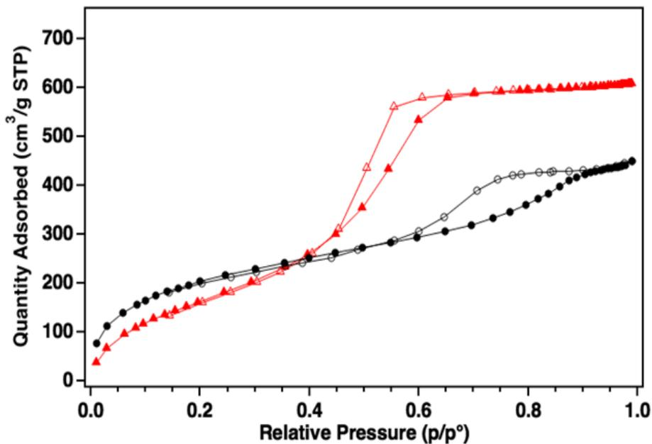
Fig. 4 N<sub>2</sub> isotherm absorption/desorption data of pSi produced (black circles) from Mg<sub>2</sub>Si and (red triangles) by anodic etching of p-type Si wafer. The line connectivity is purely for visual aid.
