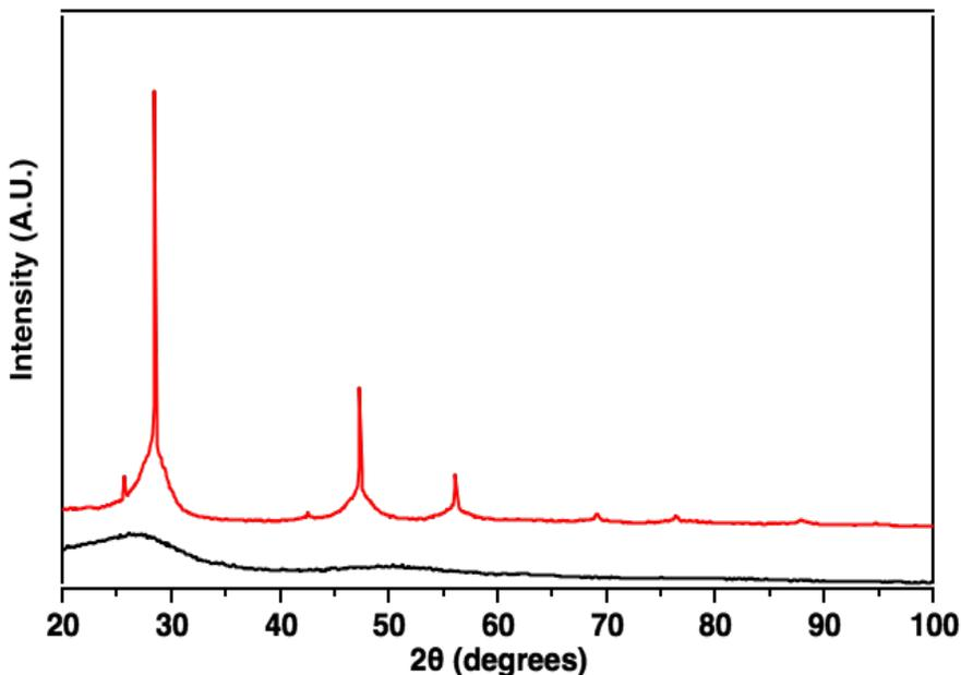
**Fig. 1** Powder XRD patterns of pSi produced (black/bottom) from  $Mg_2Si$  and (red/top) by anodic etching of p-type Si wafer
