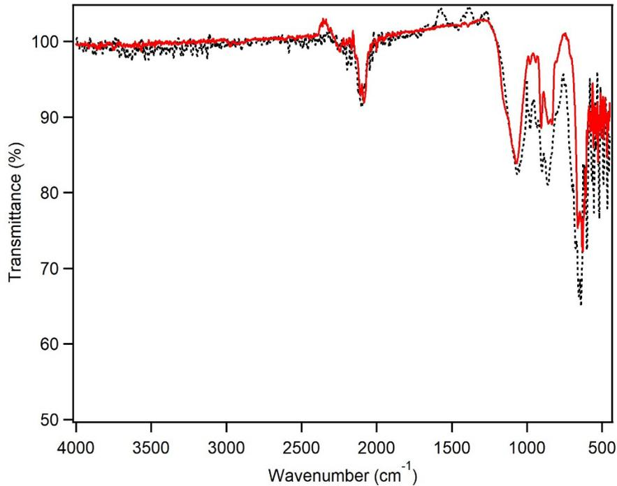
**Fig. 6** FTIR of pSi produced (black dashes) from  $Mg_2Si$  and (solid red line) by anodic etching of p-type Si wafer
