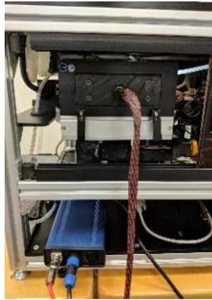
**Figure 65:** Custom-build calibration unit in use in the Applied Spectra J200 LIBS system.
