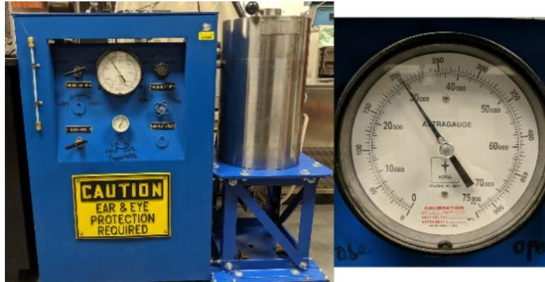
**Figure 42:** CIP cabinet with newly manufactured and installed vessel under operation at 200 MPa.
