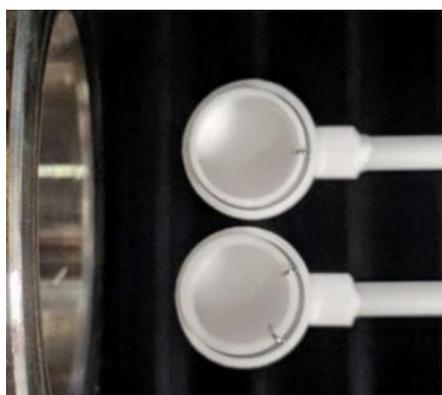
**Figure 13:** TGA crucibles pinned to back of platform with platinum wires attached to exterior wall of alumina crucible.
