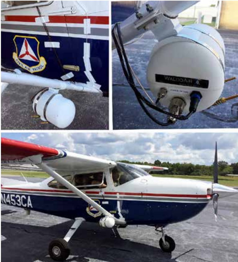
Figure 30. In 2018, CAP Cessna 182T aircraft employed specialized WaldoAir camera systems to capture multispectral imagery of damage in North Carolina caused by Hurricane Florence. (Photograph courtesy of CAP National Headquarters.)
