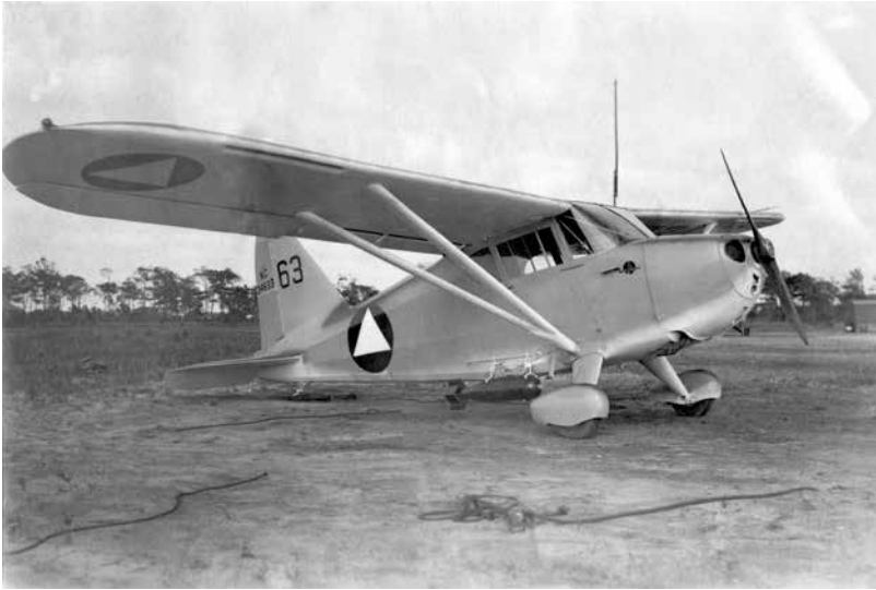
Figure 26. Stinson Voyager 10A owned by Bruce P. Ellen of Canton, North Carolina, seen at Coastal Patrol Base No. 21, Beaufort, North Carolina, in Navy three-tone camouflage, armed with a Navy Mk 15 100-pound practice bomb. (Photograph courtesy of the Charles Small Family, Richmond, Virginia, via the Morse Center.)
