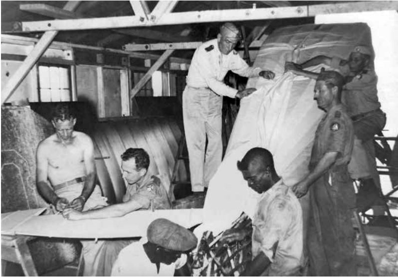
Figure 24. Personnel of Coastal Patrol Base No. 10, Beaumont, Texas, replacing the fabric covering on what appears to be a Fairchild Model 24. (Photograph courtesy of the Morse Center.)
