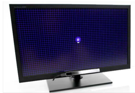
Fig. 8.12 EyeTribe tracker was tested for monitoring the eye movement
