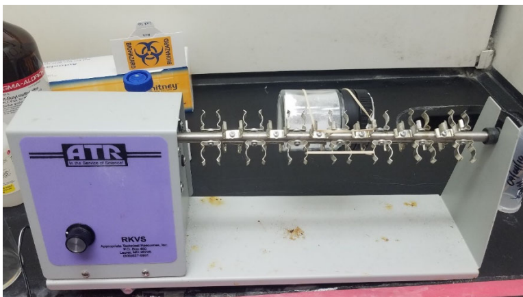
Figure 3. Dynamic TADD storage setup.
