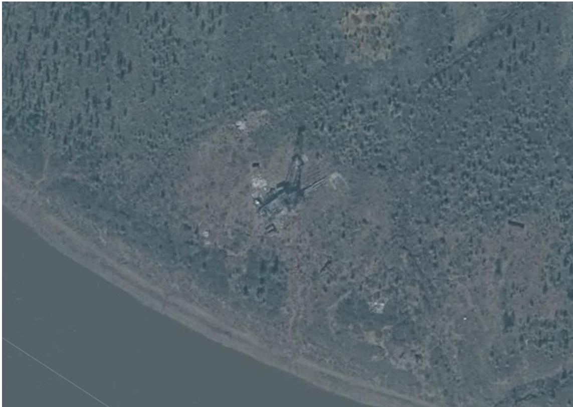
Figure 93. Satellite image from Here.com that shows the Horizon-4 PNE site and remaining infrastructure. The shadow of the emplacement tower is visible extending to the north. A slight collapse crater having a diameter of about 130 m appears visible at the site.
