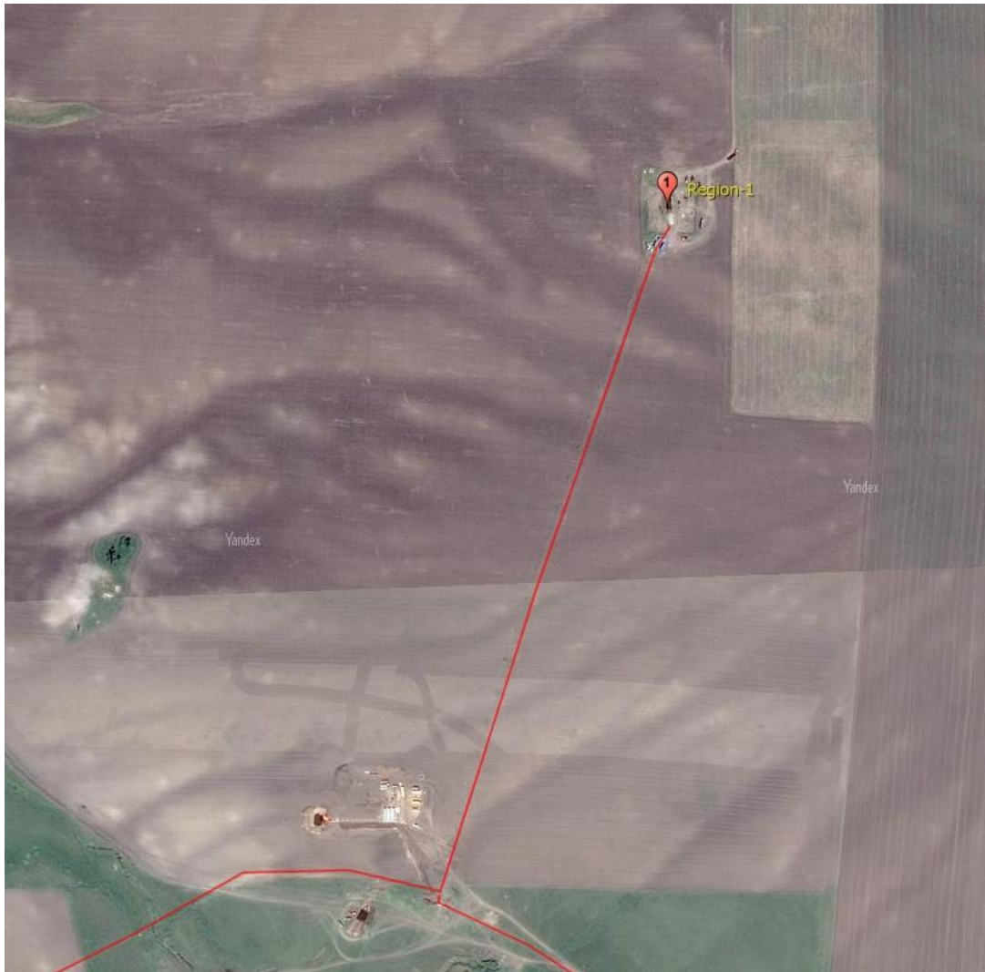
Figure 59. High resolution undated image from Yandex.ru showing active workings at the Region-1 site and a new pipeline facility with gas flare at the intersection of the East-West pipeline (red line) and spur connecting to Region-1. Based on infrastructure development, this is the most recent image available. The pipeline facility is not apparent on the Bing Maps image in Figure 56.
