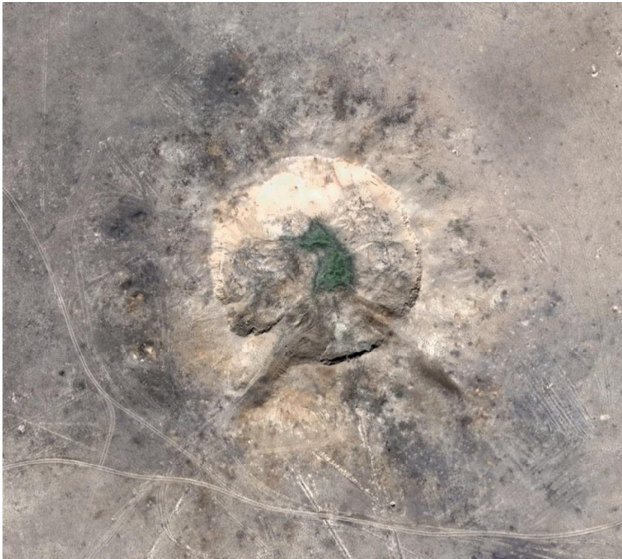
Figure 8. High resolution satellite image of the Sary-Uzen PNE excavation crater from www.maps.ovi.com . The Sultanov et al. (1999) coordinates fall on the right edge of the crater, which has a diameter of about 150 m.
