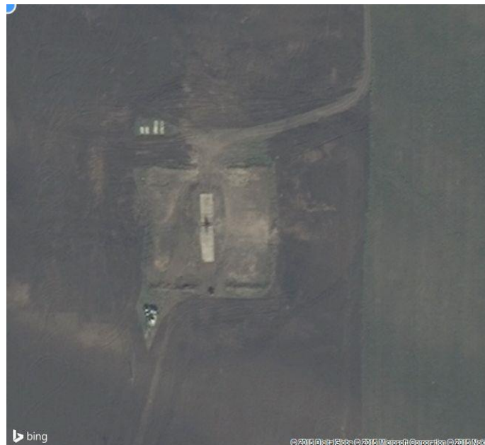
Figure 58. Newer high resolution image from Bing Maps of the Region-1 site. Fresh tracks and lack of vegetation around the borehole is indicative that the site has undergone recent development when comparing it to the Geoportal Roskozmos image in Figure 57. Utility poles and the trace of the pipeline are visible extending to the south. It is visually consistent with the Region-2 location.
