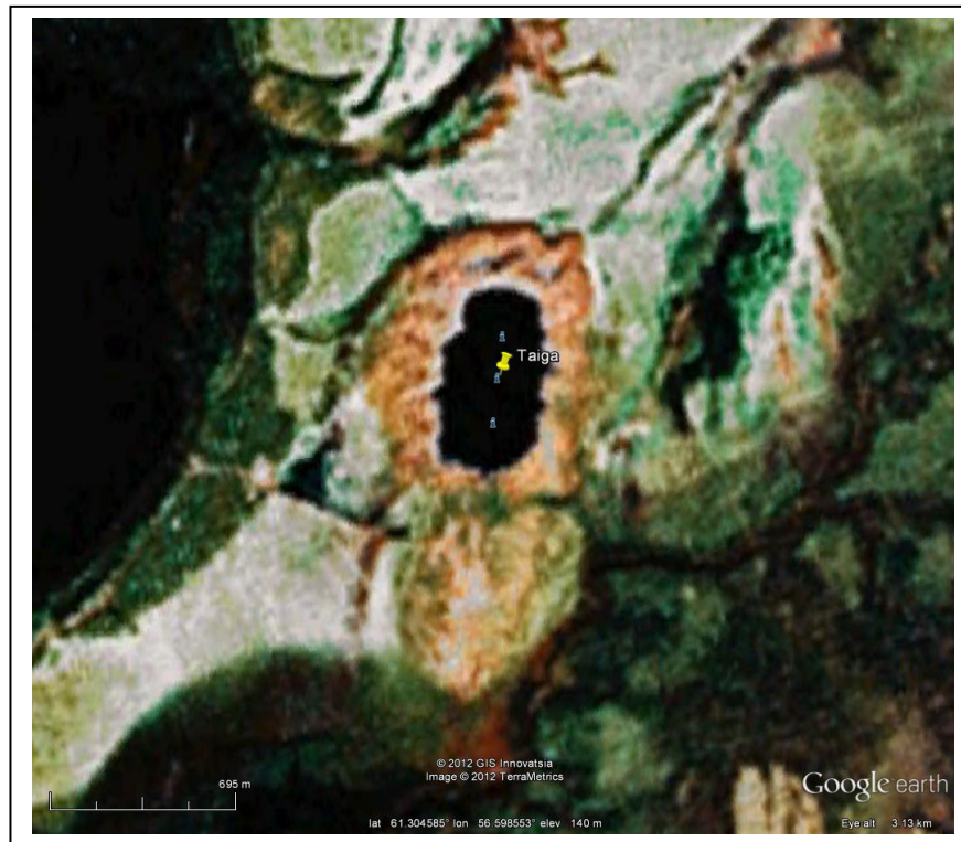
Figure 25. Excavation crater of the Taiga PNE experiment. Three 15 kt explosions were detonated simultaneously to form this lake. Image from Google Earth.
