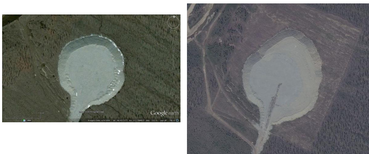
Figure 91. Satellite imagery showing the expansion of the shield covering the Crystal PNE site. The older image on the left is from Google Earth while the newer image, on the right, is from Bing Maps and shows that the shield is considerable expanded.
