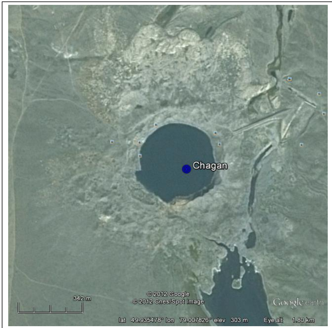
Figure 2. Google Earth image of the crater formed from the Chagan PNE. The blue point represents the coordinates as published in Sultanov et al. (1999).
