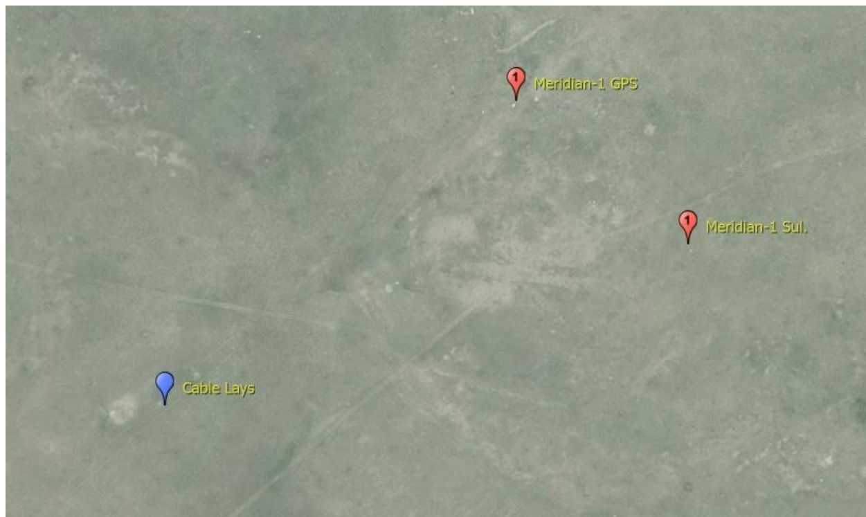
Figure 71. Overview of the Meridian-1 site from Bing Maps. The Sultanov et al. (1999) location is shown slightly to the southeast of the GPS coordinates obtained by field inspection if the site. The small white dot below the GPS location marker is the borehole. The two adjacent white dots are concrete pads probably used for erection of a support. Extending southwest from the GPS location are two parallel lines which are probably cable trenches for signals to the experiment control site.
