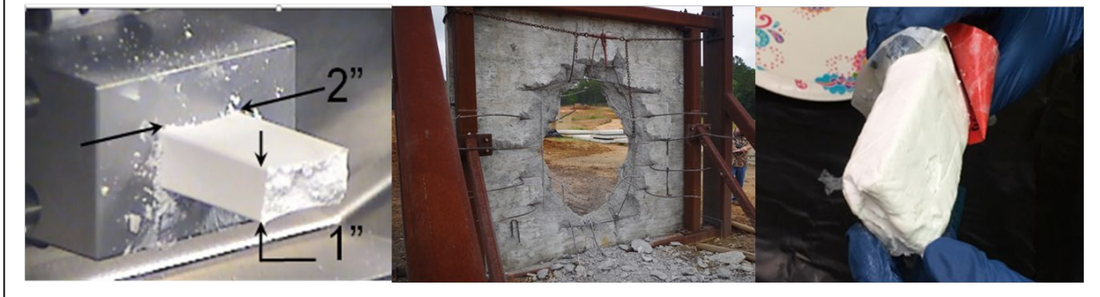
Figure 27 (U) Twin Screw Extruded PAX-52 M112 Demolition Blocks The image on the left shows PAX-52 extrudate with a near net shape of the M112 demolition block. Side concavities were designed into the inverted die to compensate for material swell upon release from the die constraint. The middle image shows a breached wall target that was defeated with PAX-52 M112 demolition blocks. No formal test plan or report of the test was provided. The image on the right shows the only remaining PAX-52 material from the TSE trial. The PI opened the M112 packaging to find the material very smooth and hand-moldable.
