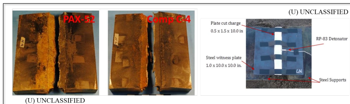
Figure 29 (U) Results of Plate Cutting Test To evaluate the energy output of PAX-52, a plate cut test was performed on 1 in. thick ASTM A36 grade 1018 steel plate. The charges for this test were cut from hand-packed M112 size charges to the dimensions of 0.5 in. x 1.5 in. x 10.0 in. The charge was placed in the center of the plate and secured with tape at each end (top right.) Five of five shots with PAX-52 completely cut the steel witness plate comparable to two baseline shots using Composition C4 (20).
