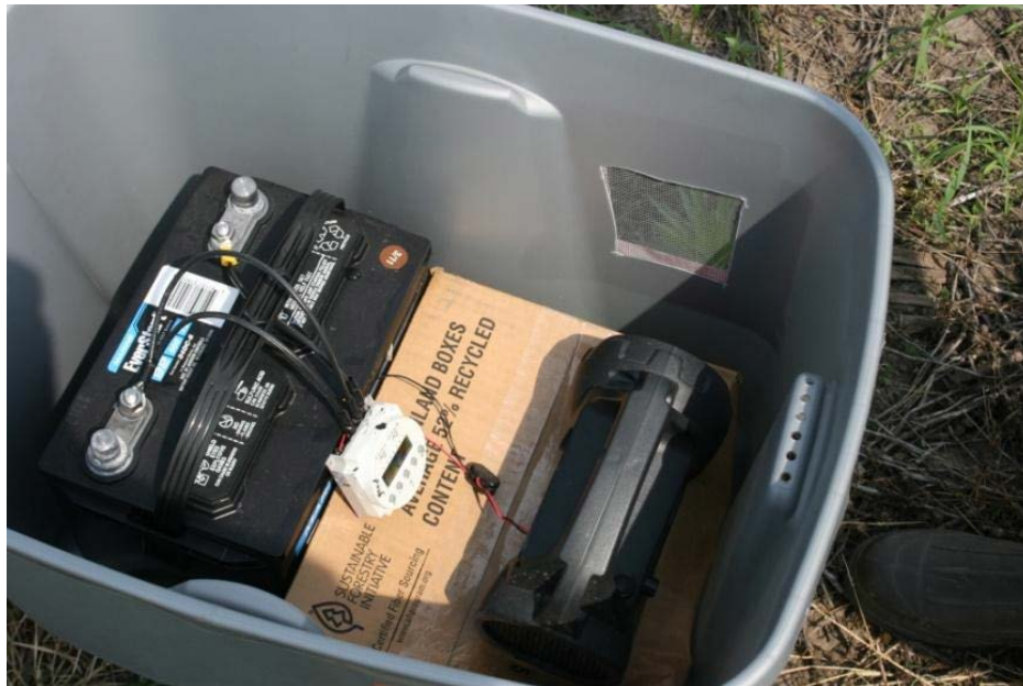
Figure 1. Call box, timer, and battery used to broadcast calls for conspecific attraction.
