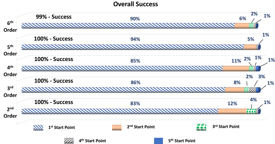
Figure 5.7: Percent successful retrievals when three targeted \alpha planes and five random starting sets of phase values are permitted (noiseless).
