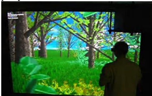
Figure C-2-8. Perspective in VR matches that of the user in the virtual world.
