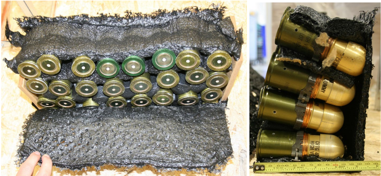
Figure 8 Post-test 1 remains; inert 40-mm slow heating
