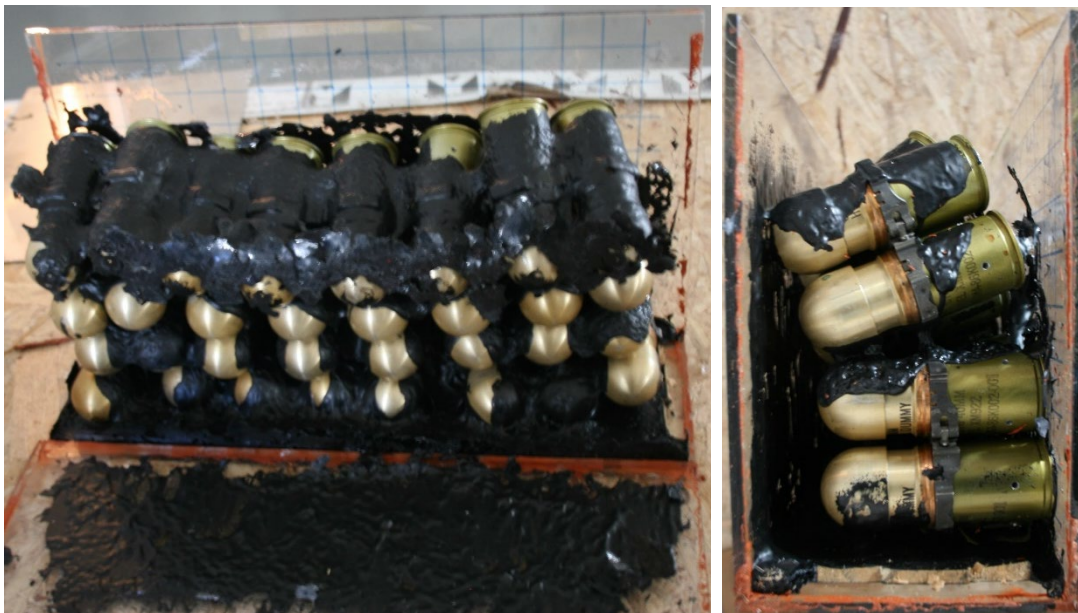
Figure 9 Post-test 2 remains; inert 40-mm slow heating
