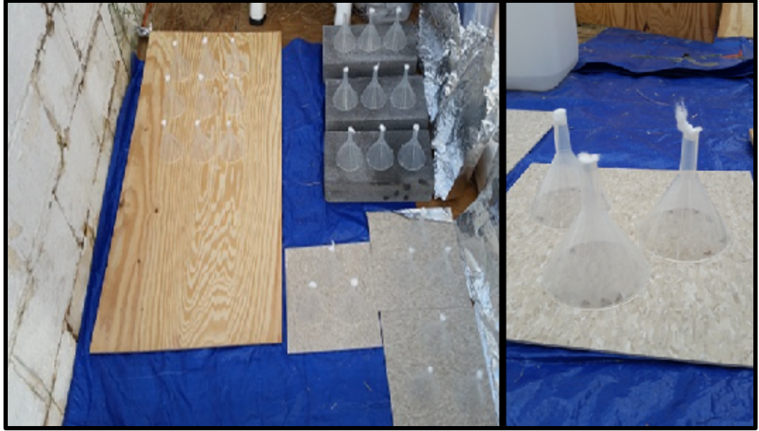
Figure 13. Cone assays performed on three different surface materials for three exposure periods.
