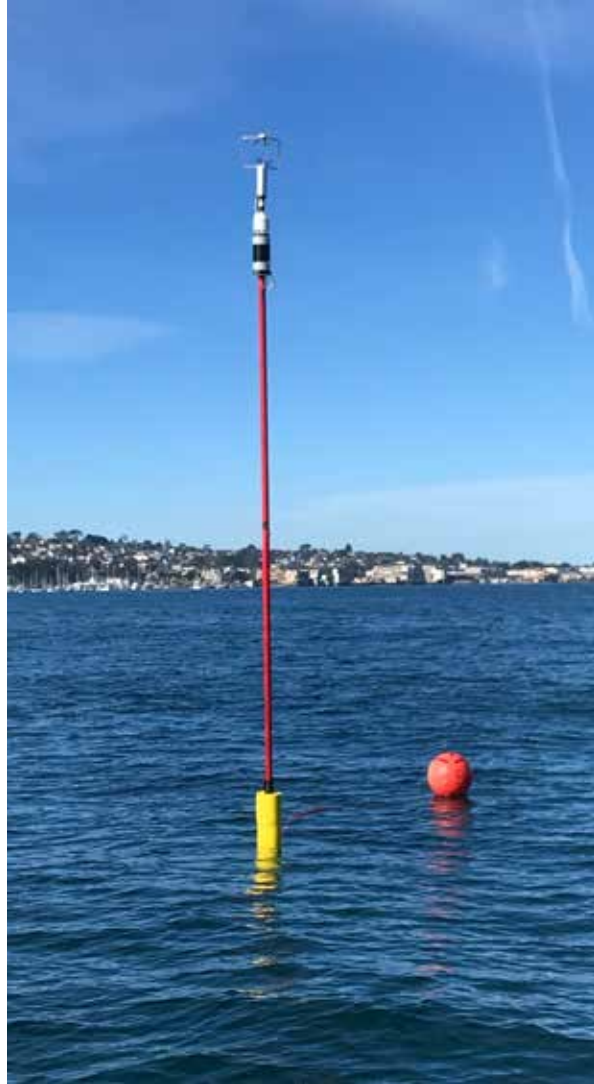
Figure 4. A picture of the prototype I-SPAR and its mooring float deployed off Del Monte Beach, Monterey Bay, California. Taken on 10 January 2020, the image shows the 5 m subaerial portion of the buoy from the electronics module (Figure 2a) at the top to the flotation cylinders at MSL.
