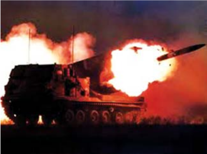
Figure 5.3. US Field Artillery Multiple Launch Rocket System (MLRS) conducting fire mission. Photo courtesy of Morris Swett Digital Collections & Archives, Fires Center of Excellence, Fort Sill, Oklahoma.
