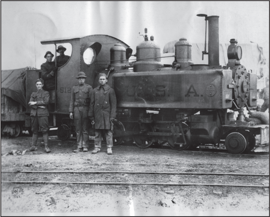
Figure 7.4 Although narrow gauge (60cm) railroads, such as this one near Rattenhout, were invaluable for the Meuse-Argonne Offensive, they still could not carry enough to eliminate the need for trucks and wagons, moving over miserable roads. This engine was made by Baldwin Locomotive. Photo taken 28 October 1918, as the American logisticians took advantage of the tactical pause to push supplies forward. Photo courtesy of the US Army Quartermaster Museum.
