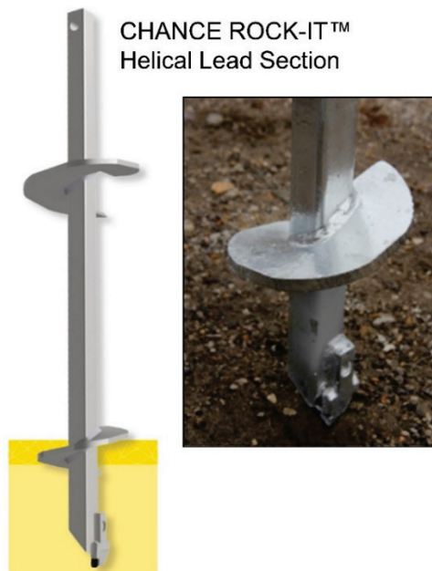
Figure 63. Chance ROCK-IT™ helical lead section designed to penetrate rocky soils.
