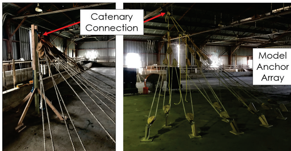
Figure 14. Models of anchor array connections using tension-distributing pulley arrangements.
