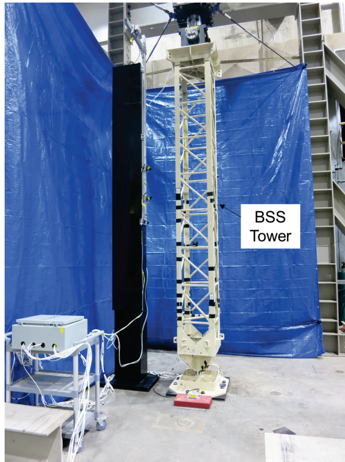
Figure 31. Fully assembled BSS tower.
