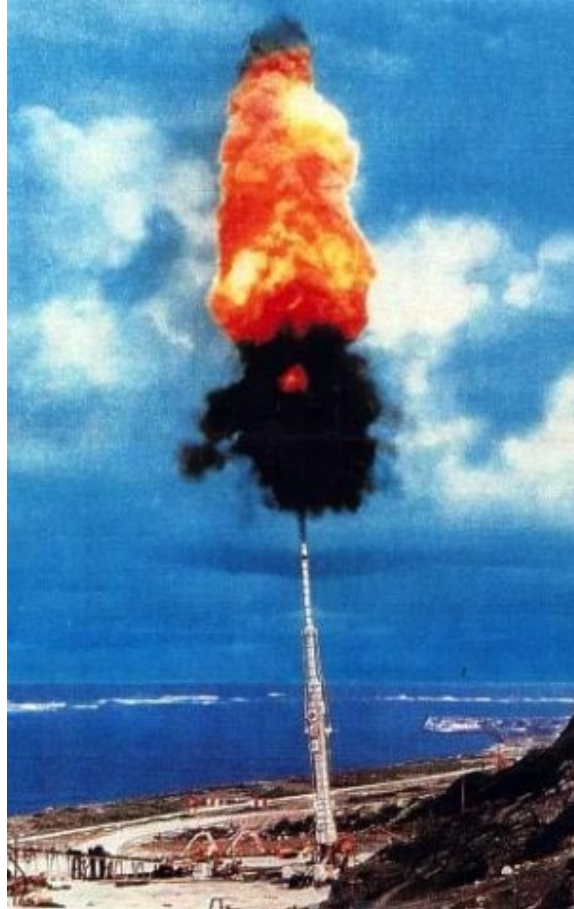
Figure 4. 16.7 Inch (42.4 Centimeter) L86 HARP Barbados Gun Firing at 85° Elevation
