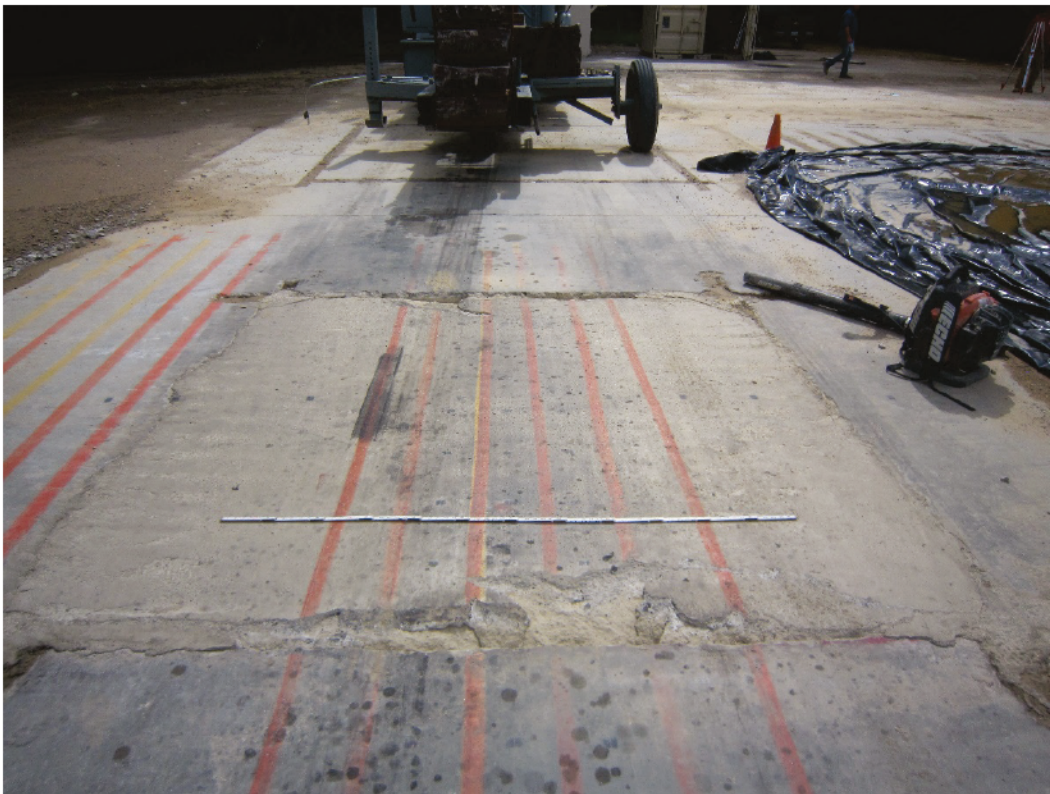
Figure 4.6. Post-traffic photographs of Repair 4 after 830 passes.
