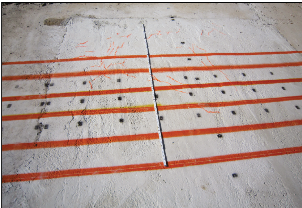
Figure 4.11. Shrinkage cracks on Repair 4.
