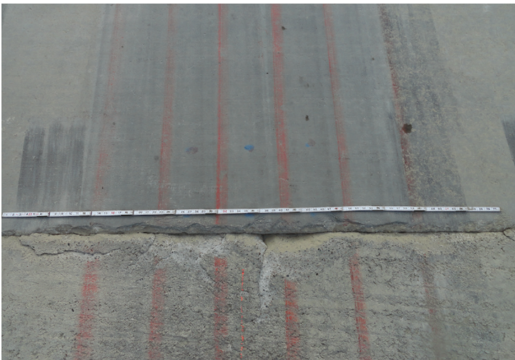
Figure 4.9. Post-traffic photographs of Repair 7 after 1,792 passes.
