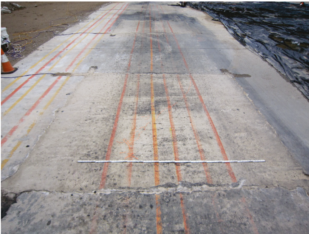
Figure 4.4. Post-traffic photographs of Repair 2 after 3,600 passes.
