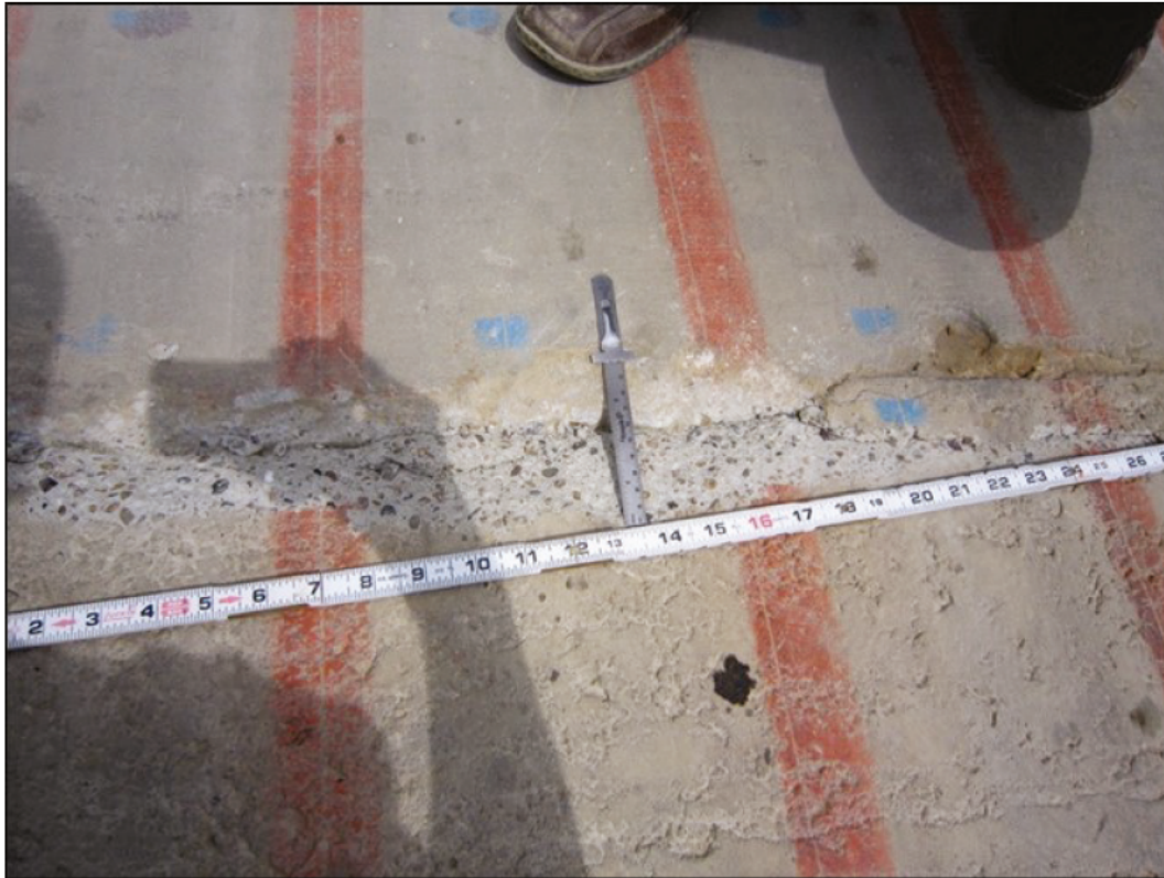
Figure 3.40. Measuring a spill on repair edge.
