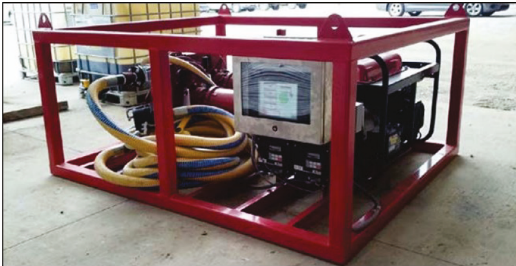
Figure 3.20. CRADR 1-L prototype foam dispensing system.
