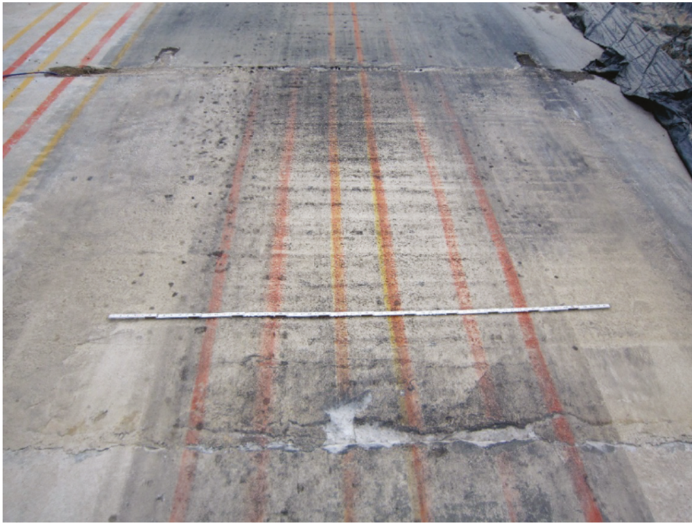
Figure 4.4. Post-traffic photographs of Repair 2 after 3,600 passes.
