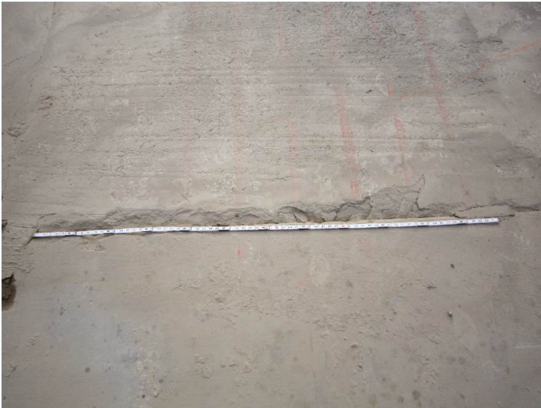
Figure 4.7. Post-traffic photographs of Repair 5 after 1,520 passes.
