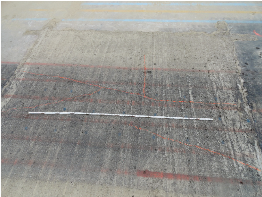
Figure 4.9. Post-traffic photographs of Repair 7 after 1,792 passes.
