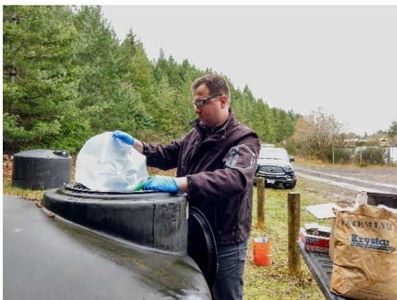
Figure 6. Adding <sup>13</sup>C-, <sup>15</sup>N-labeled RDX to PPT tank
