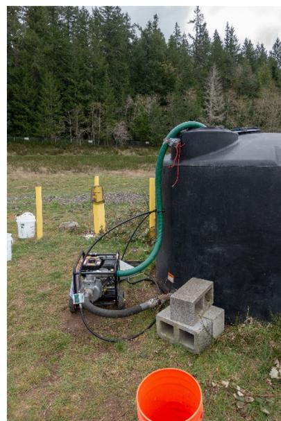
Figure 5. Recirculation pump mixing PPT injectate
