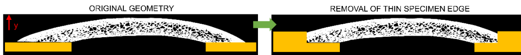
Fig. 26 Illustration of skullcap specimen with thin specimen edge removed. The skullcap shown here is from LR03.
