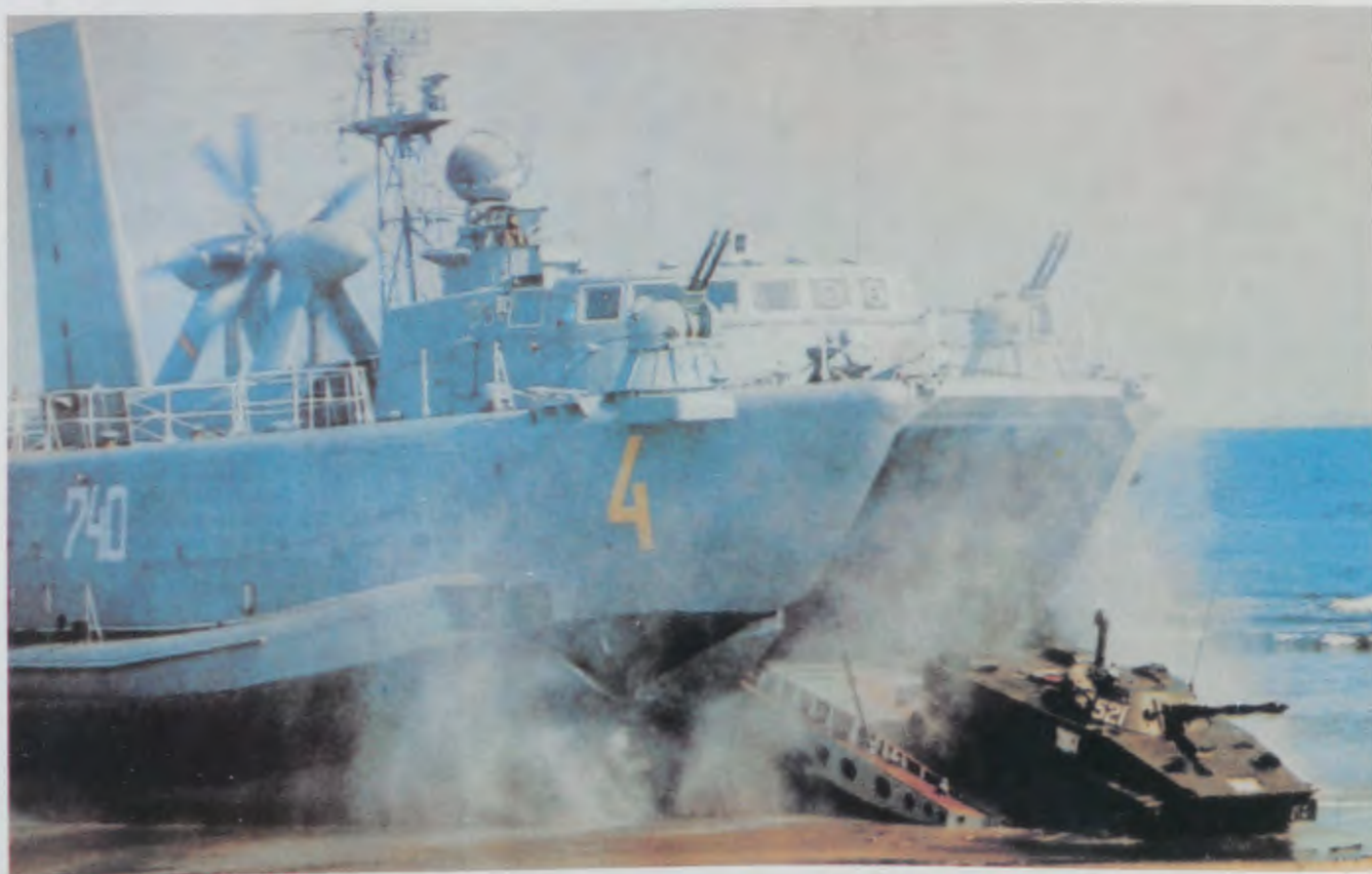
The AIST is the world's largest operational air cushion vehicle. Its 250-tons displacement, aircraft-type gas-turbine main propulsion, and bow and stern ramps facilitate Soviet amphibious force delivery.
