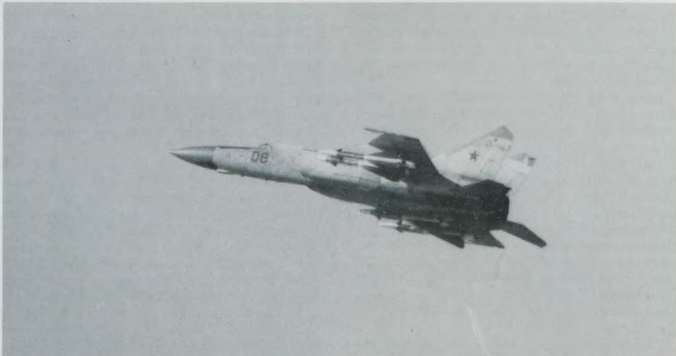
The MiG-25/FOXBAT E interceptor, above, has a limited look-down/shoot-down capability. Acquisition of Western technology enabled the USSR to fit the MiG-31/FOXHOUND interceptor with a true look-down/shoot-down radar system.
