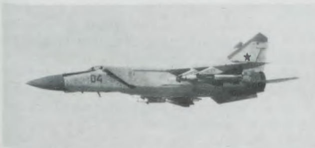
A new generation of air defense, all-weather interceptors is joining the highly capable FLOGGER G, seen at top with AA-7 and AA-8 air-to-air missiles under wing, and FOXBAT E, seen with the AA-6 missile.
