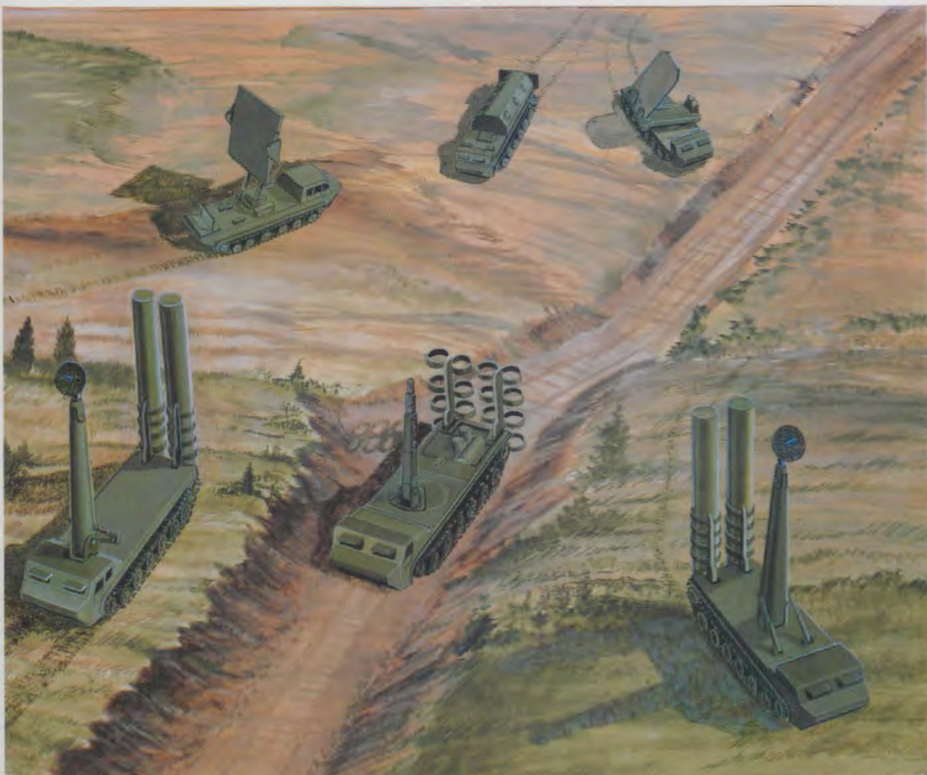
The surface-to-air missiles of the SA-X-12 air defense system are designed to counter high performance aircraft and will also have a capability against tactical ballistic missiles.
