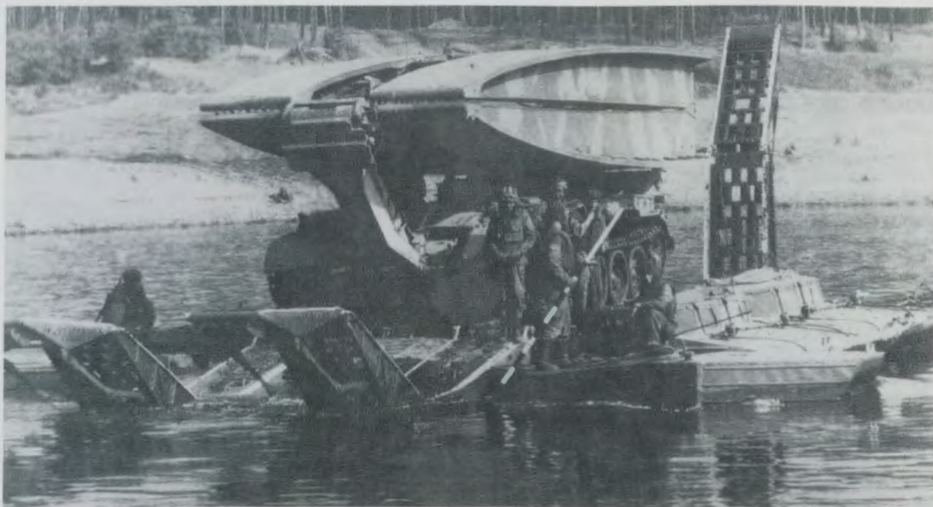
In the 1980s, Soviet ground forces have fielded a new bridge/ferry system to augment their river-crossing capability; here, a heavy amphibious ferry transports a tank-mounted scissors bridge.
