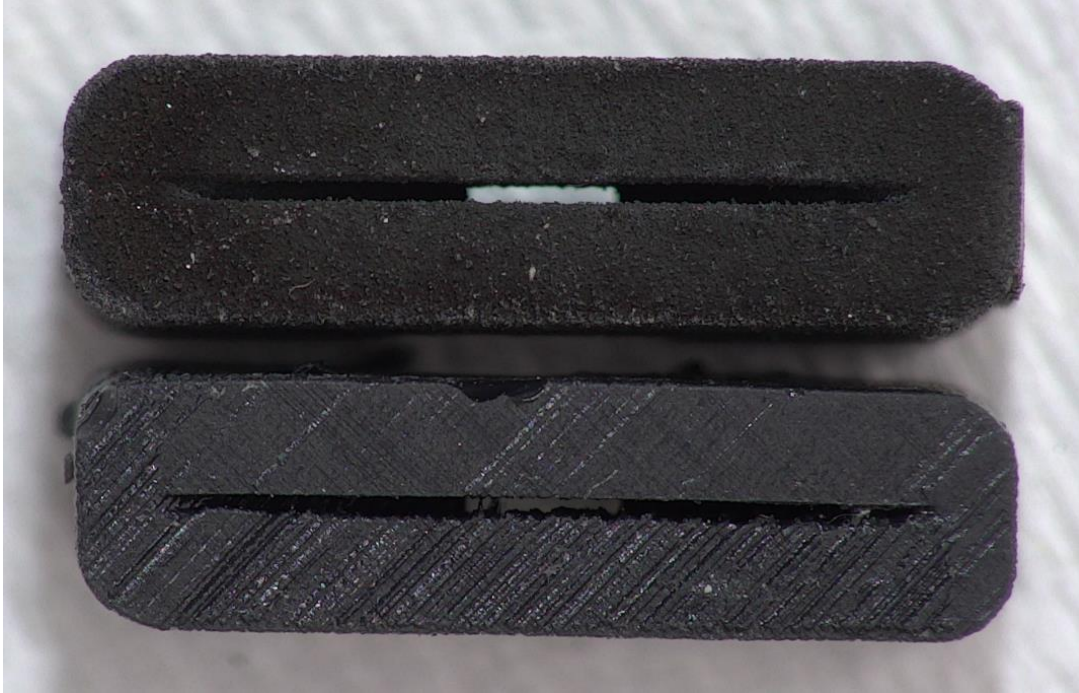
Figure 14 3D-printed solar sensor slit comparison: top - single-piece metal with scale/bottom - single-piece plastic
