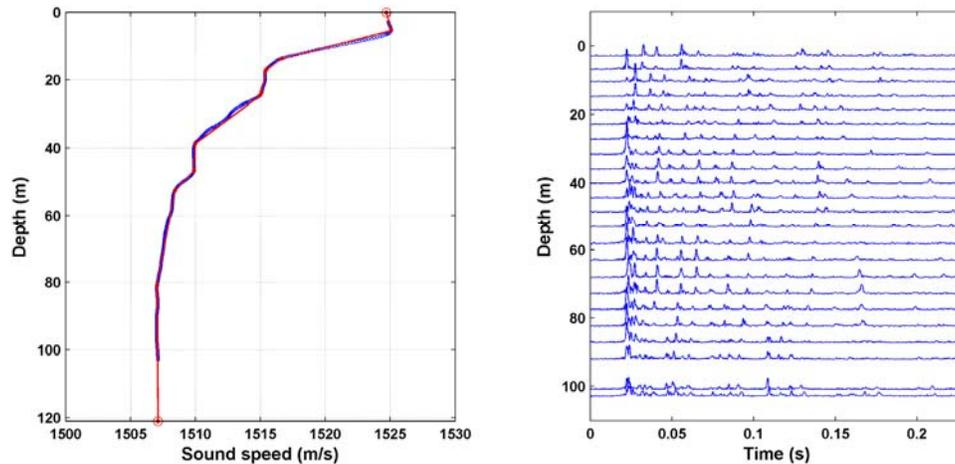
**FIGURE 4.** Left) sound speed profile collected by glider Greta, and Right) time series of acoustic pulses collected by glider Greta at the same time.
