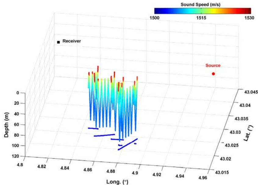
FIGURE 2. The sound speed measured at the positions (coordinates and depths) of glider Greta on Sep. 18, 2012
