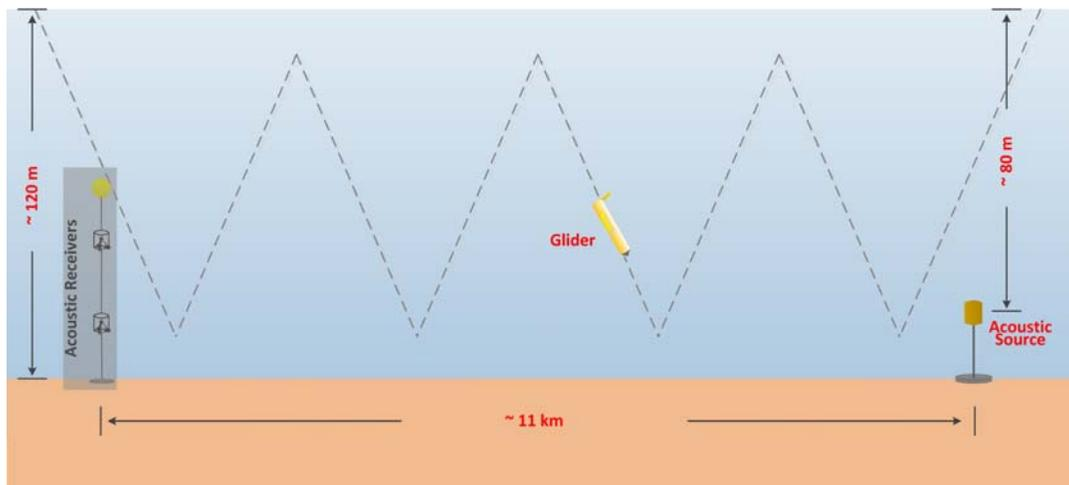
FIGURE 1. Side view of the glider track with respect to the acoustic source.
