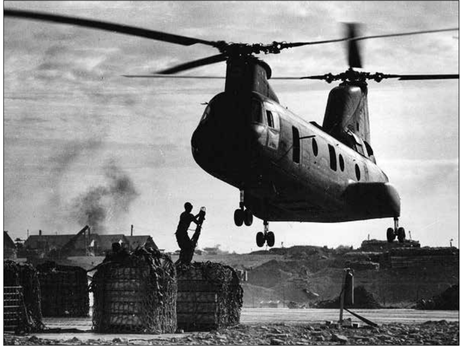
Photo by Maj Barry Broman, USMCR (Ret) Boeing Vertol CH-46 Sea Knight helicopter at An Hoa Combat Base preparing to take an external load of supplies to be flown to 5th Marine units in the field.
