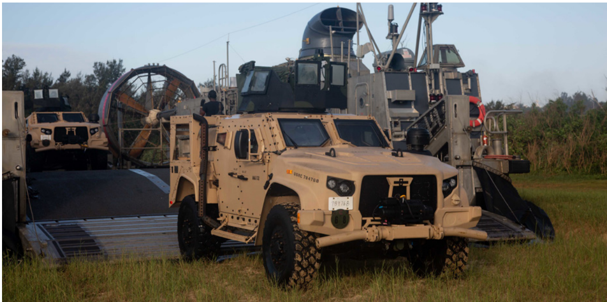
U.S. Marines offload joint light tactical vehicles from a U.S. Navy air cushioned landing craft in Okinawa, Japan during exercise Noble Fury 21. (USMC photo by Lance Cpl. Kolby Leger)
