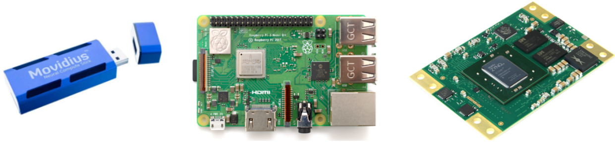
Fig. A1—The hardware we applied our deep learning models on: Neural Compute Stick, ARMv7 (Raspberry Pi), and Xilinx Zynq 7045 (SoC) FPGA respectively.
